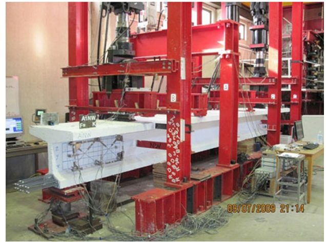
Fig. 4 Test set up for girders.
