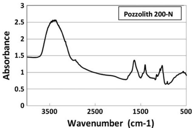
Fig. 2 Typical absorbance versus wavenumber spectra for admixture Pozzolith 200-N.
