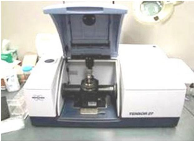
Fig. 1 The IR spectrometer used in this study.
