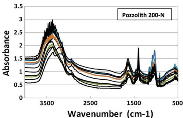
Fig. 3 Absorbance versus wavenumber spectra for all 12 scans from three different batches of admixture Pozzolith 200-N.
