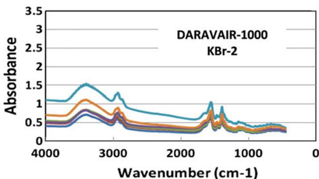
**Fig. 5** IR scan of admixture *Daravair-1000* using KBr-2.
