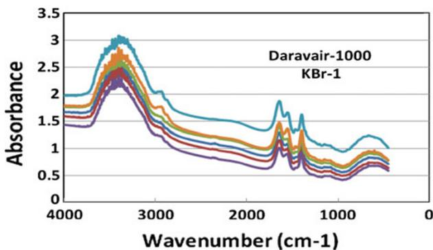
**Fig. 4** IR scans of admixture *Daravair-1000* using KBr-1.
