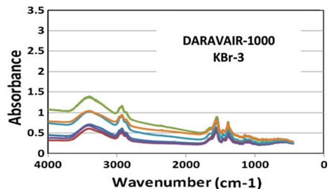
**Fig. 6** IR scans of admixture *Daravair-1000* using KBr-3.
