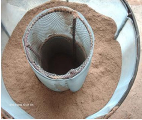
Fig. 1 The incinerator with rice husk.
