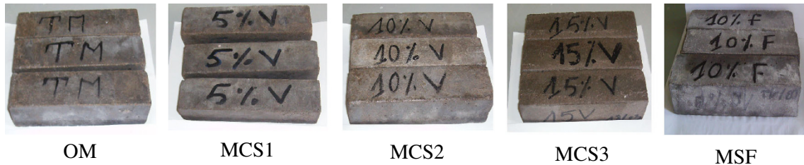
Fig. 11 State of the samples after 60 days of immersion in Na 2 SO 4 .
