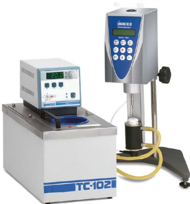
**Fig. 3** Rheometer for the measurement of rheological properties of mortar and cement paste.
