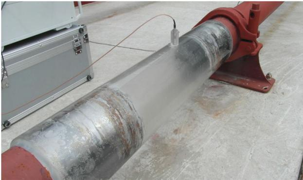
**Fig. 5** Application point of the UVP and transparent engineered plastic.
