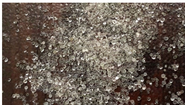
Fig. 3 Glass beads used as a fine aggregate to reduce the temperature gradient in concrete sample.
