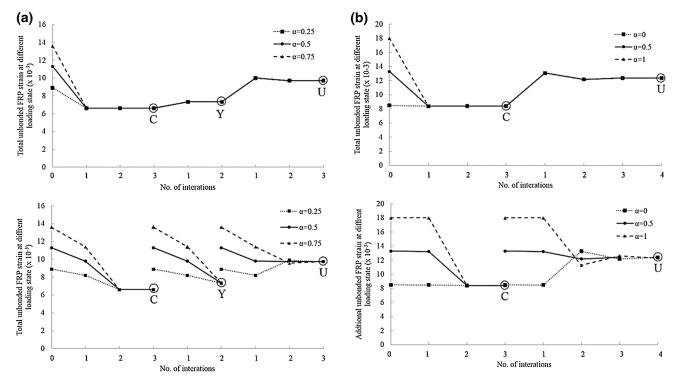
Fig. 4 Examples of convergence trend of the model prediction with two different ways:  $\alpha$  in Eq. (12a) given in the initial cracking state only; and the same  $\alpha$  assigned at the beginning stage of each state. **a** RU50. **b** TO45.
