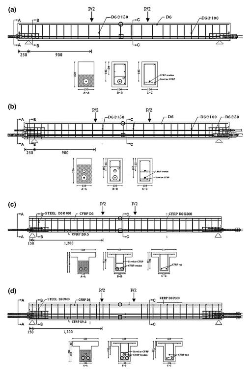
Fig. 5 Beam specimens ("*open circle*" for concrete strain gages and "*open square*" for unbonded CFRP tendon strain gages). a RU50, RU70, or RO55. b RO50. c TB45. d TO45.
