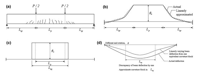
Fig. 2 Approximation by one equivalent curvature block. a Beam under 4-point loading. b Actual and linearly approximated curvature distributions. c One equivalent curvature block. d Deflection of the beam under the assumption of one equivalent curvature block.
