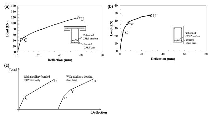
Fig. 1 The experimentally observed and theoretically modeled load-deflection *curves* of the internally unbonded CFRP prestressed concrete beams. a Beam specimen TB45. b Beam specimen RU50. c Characteristic points in theoretical load-deflection modeling (not to scale).
