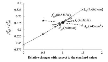
**Fig. 10** Relative effects of parameters on  $\rho_{pfb}^U / \rho_{pfb}^B$  (Values in *parenthesis* represent standard ones in Table 5).
