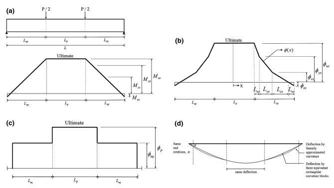
Fig. 3 Moment, curvature distributions and deflections at ultimate state. a Moment distributions. b Linearly approximated curvature distributions. c Three equivalent rectangular curvature blocks. d Close approximations of beam deflection and rotation at support by three equivalent rectangular curvature blocks to those by linearly varying curvatures.
