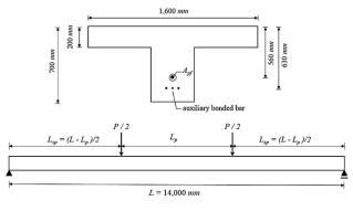
Fig. 7 Standard beam for parametric studies.
