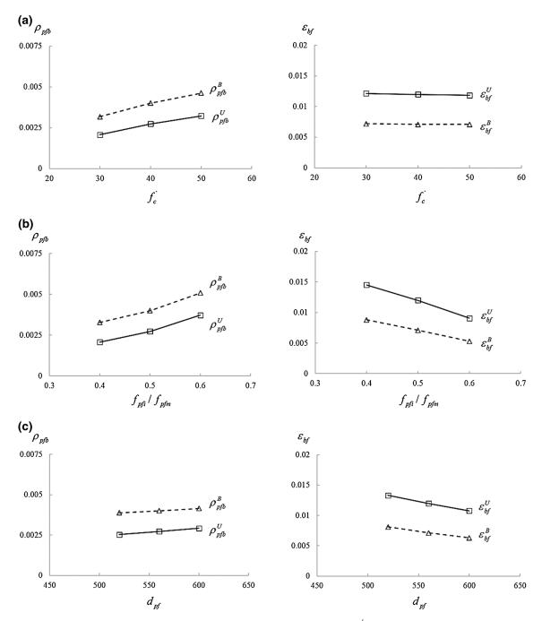
Fig. 9 Effects of main parameter on  $\rho_{pfb}$  and  $\varepsilon_{bf}$ . a Concrete compressive strength  $(f'_c)$ . b Initial prestress  $(f_{pfi}/f_{pfm})$ . c Effective depth  $(d_{pf})$ . d Amount of bonded rebar  $(A_{bf})$ . e Relative distance between loading points,  $L_p/L$ .
