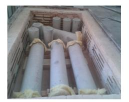
Fig. 2 Sample arrangement of test specimens in electric furnace.
