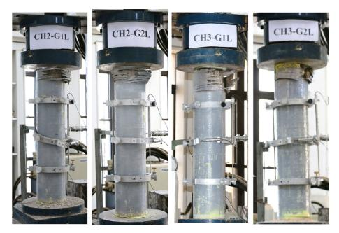
Fig. 8 Failure modes for GFRP wrapped specimens.
