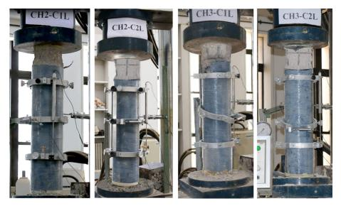
Fig. 7 Failure modes for CFRP wrapped specimens.
