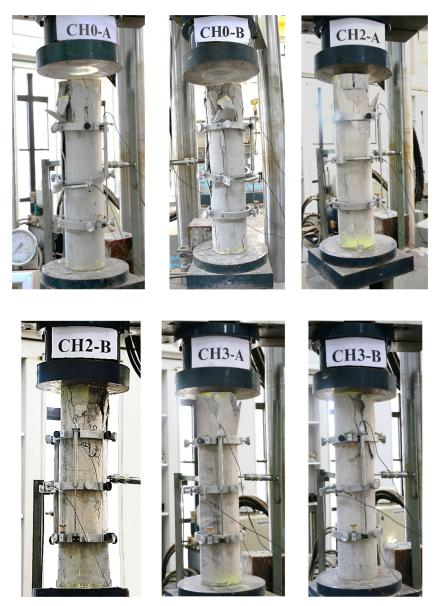
Fig. 6 Failure modes for control specimens.
