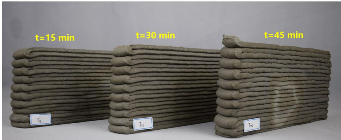
Fig. 3 Structures constructed by the proposed tailing concrete at different paste ages.
