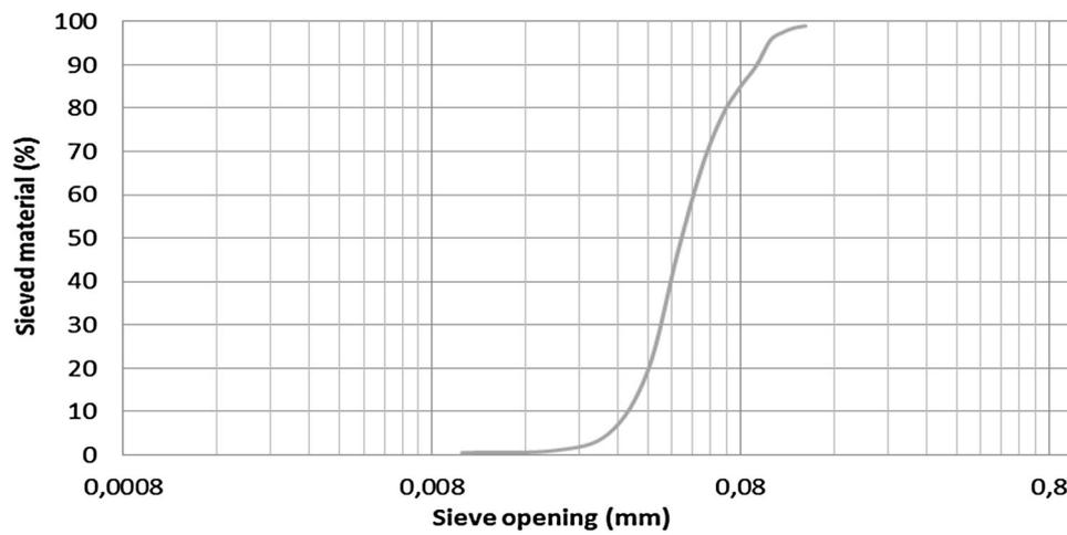
Fig. 5 Granulometric (grain-size) curve of mud.
