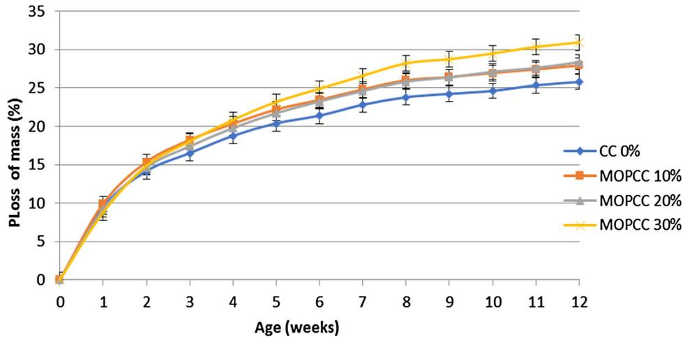
Fig. 10 Mass loss of concretes aged 90 days and immersed in H<sub>2</sub>SO<sub>4</sub> solution.
