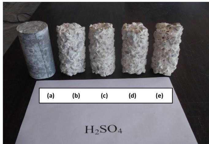
Fig. 11 Aspect of healthy concrete and attacked by the sulfuric acid solution: a concrete not attacked, b CC 00%, c MOPCC 10%, d MOPCC 20%, and e MOPCC 30%.
