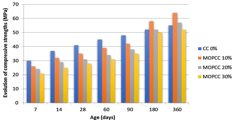
**Fig. 8** Compressive strength of concretes in MPa, as a function of time.
