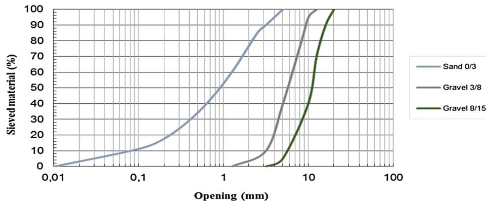
**Fig. 6** Grain size distribution curves of aggregates.
