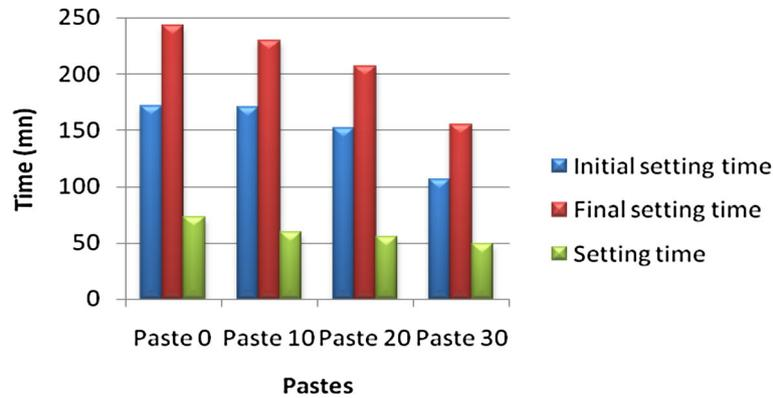
**Fig. 7** Influence of mud content on the setting time.
