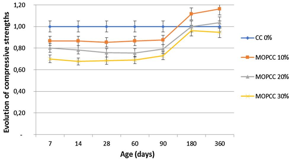
Fig. 9 Evolution of the strength of mud-based concretes with respect to control concrete.
