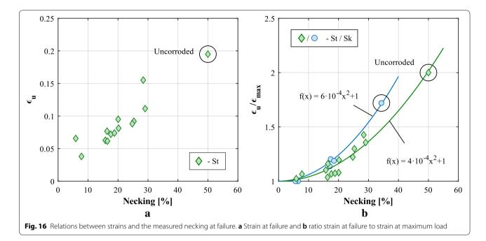
from the weak trend found in Fig. 14a is that the remaining cross-sectional area in the bar is not the only factor governing the reduction in strain capacity  $\varepsilon_u$  or  $\varepsilon_{max}$  and the loss of necking. In order to investigate whether the shape of the pit could play an important role in the behaviour of the  $\varepsilon_u$  or  $\varepsilon_{max}$  and the necking of the bar at failure, the following pit shape factor,  $\psi$ , was defined:
