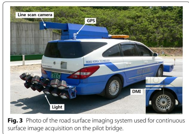
was driven at an average speed of 80 km/h to collect the images of the road surface of all lanes that includes the shoulders. The location and areal extension of deteriorations from various sources were calculated by using an image-processing computer program.
