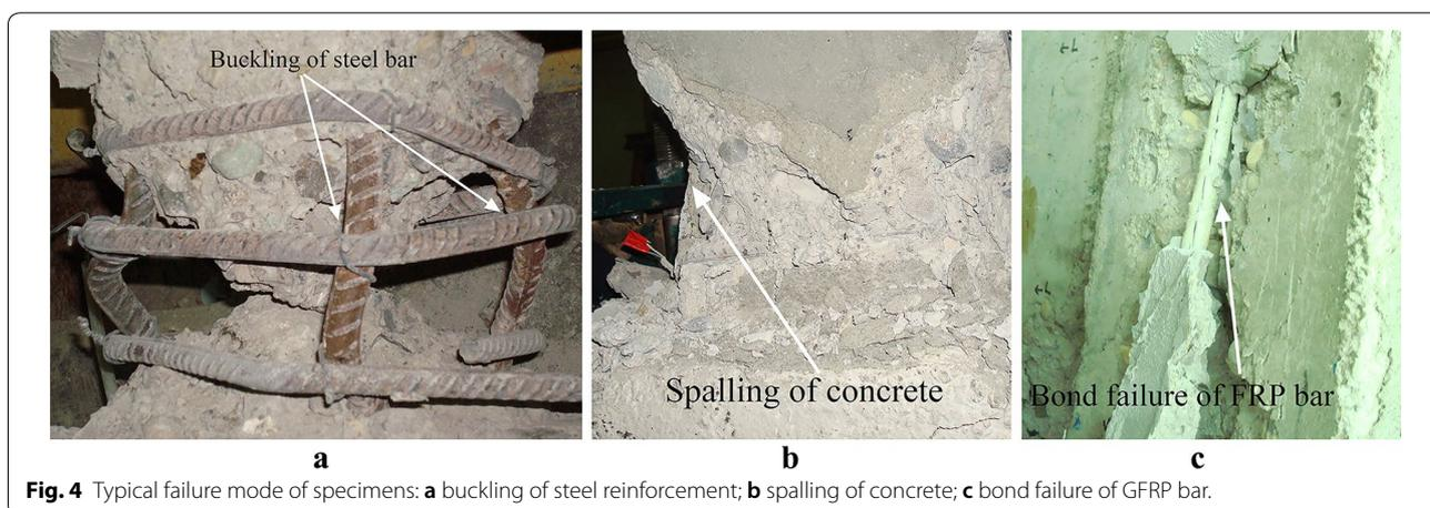
displacement of 19.8 mm, the first steel rebar started to yield. The lateral strength reached the peak value at the displacement of about 20.6 mm. The failure of the epoxy paste happened at the displacement of 35.6 mm. The failure process included the development of splitting cracks in the epoxy paste, and bond failure of GFRP bars followed by concrete crushing at the column base. In this time, the load sharply decreased.
