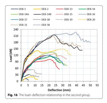
exhibits a decline and rather steeply. On the other hand, for the DEB-15, DEB-14, and DEB-16, their softening effect was more dominant compared to the DEB-3 and DEB-13. However, the DEB-15 exhibits the ability to perform more plastic deformation up to failure compared to other beams.
