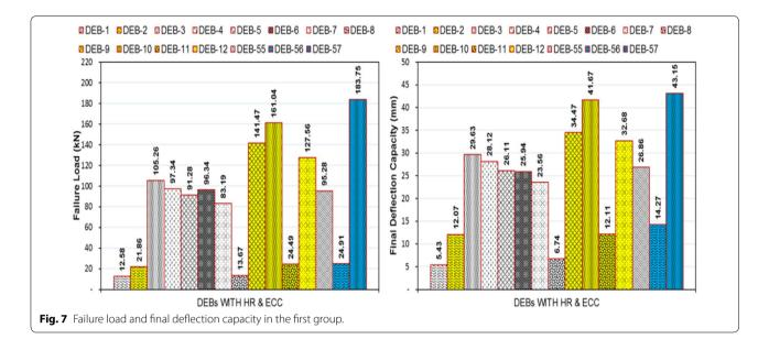
of the DEB-7 was much higher compared to the DEB-8, which had a failure load of 508.56% and deflection capacity of 249.55%. In fact, as occurred at the DEB-8, it has exhibited that the HR cannot act alone to resist the shear force in the dapped-end region. However, at least the NFR or NHR should be involved together with the HR in resisting the shear force in the dapped-end region.
