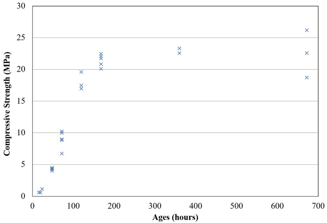
**Fig. 5** Compressive strength with ages (30 MPa)
