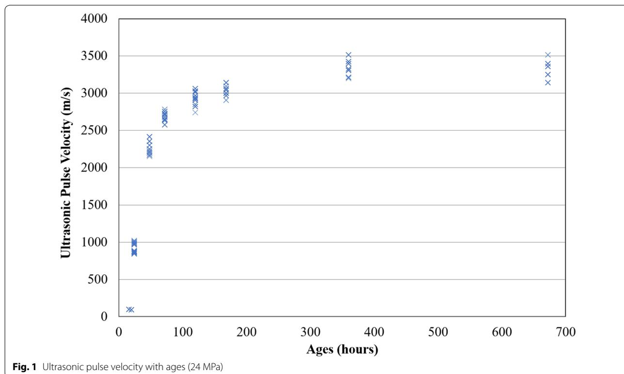
**Fig. 1** Ultrasonic pulse velocity with ages (24 MPa)
