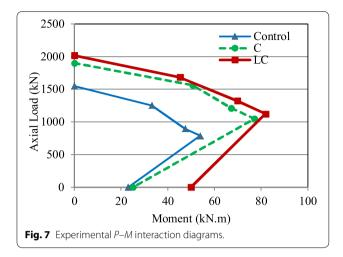
specimens tested under compression loading at 0, 0.13*D*, 0.26*D*, 0.34*D* loading eccentricities and in pure bending, i.e. at infinite eccentricity.
