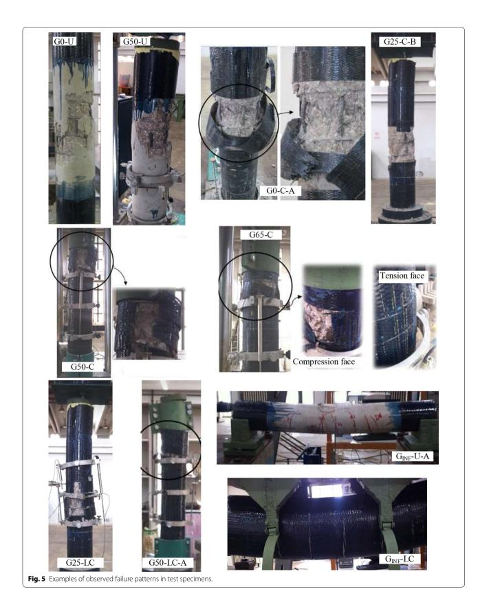
Post inspection of the FRP jackets confirmed proper lamination of the FRP sheets. Examination of the FRP sheets at locations of rupture revealed that a thin layer of concrete was attached to the inner surface of the sheets thereby indicating proper bonding and thus full activation of the fabric sheets. Adequacy of the adopted overlapping system was confirmed during the tests. Delamination of the FRP sheets was not observed at the overlapping zones.
