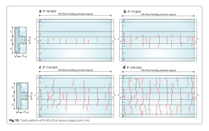
were gradually pulled out, leading to the crack localization with significant increase of crack width. It is because of the local bond failure between fiber and the UHPC matrix as well as rebars yielding. When the applied load approached to the peak load of the specimen, the crack localization with excessive crack width (i.e. higher than 4 mm) and rebars yielding was observed, and thus the specimen was regarded as failure in this investigation.
