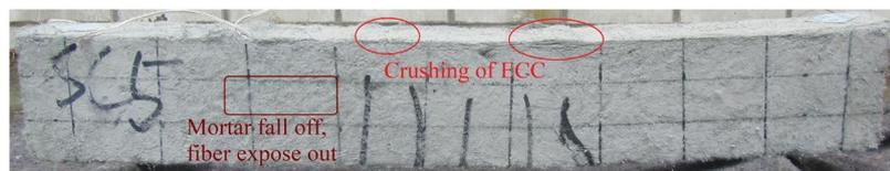
Fig. 8 Failure modes of selected test specimens.
