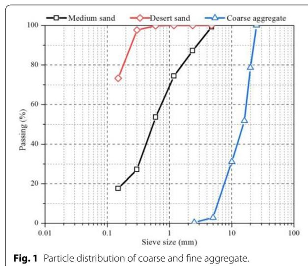
**Fig. 1** Particle distribution of coarse and fine aggregate.
