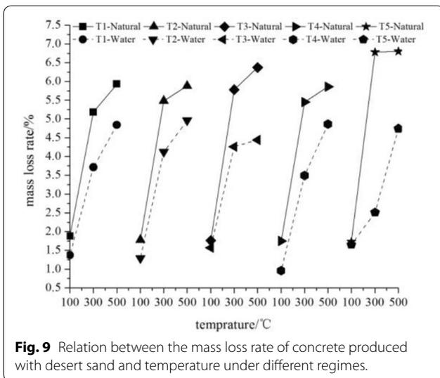
**Fig. 9** Relation between the mass loss rate of concrete produced with desert sand and temperature under different regimes.
