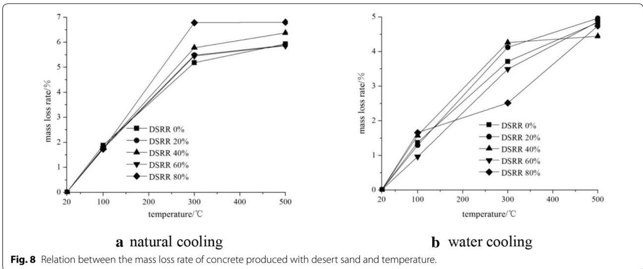
**Fig. 8** Relation between the mass loss rate of concrete produced with desert sand and temperature.
