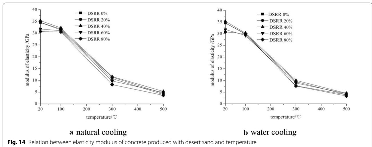
**Fig. 14** Relation between elasticity modulus of concrete produced with desert sand and temperature.
