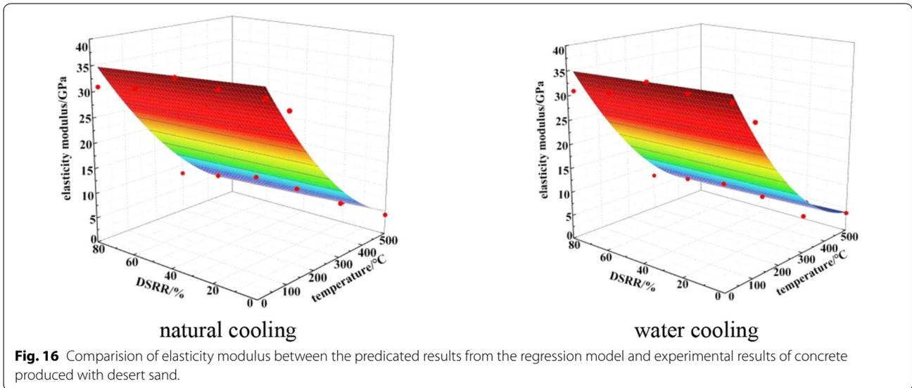
$$\frac{E_c(t, s)}{E_c} = 1.0597 + 0.01855s - 2.22002 \left( \frac{t - 20}{700} \right) + 1.21061 \left( \frac{t - 20}{700} \right)^2 \quad (6)$$
