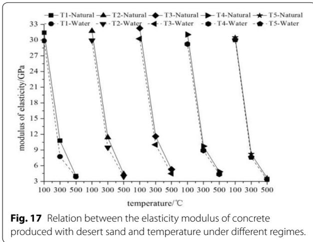
**Fig. 17** Relation between the elasticity modulus of concrete produced with desert sand and temperature under different regimes.
