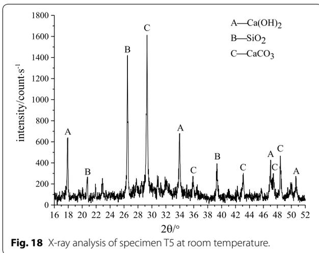
**Fig. 18** X-ray analysis of specimen T5 at room temperature.
