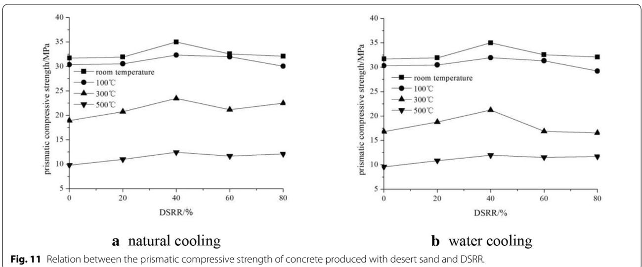
concrete produced with desert sand after elevated temperature increased firstly, and then declined with DSRR, the maximum value of which was obtained when DSRR amounted to 40%.
