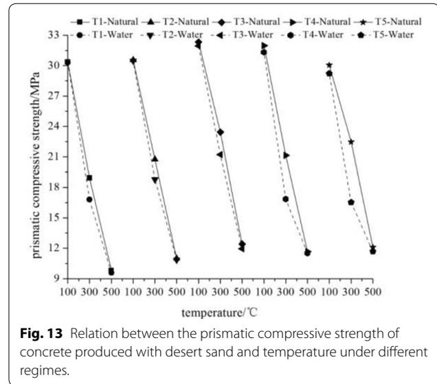
**Fig. 13** Relation between the prismatic compressive strength of concrete produced with desert sand and temperature under different regimes.
