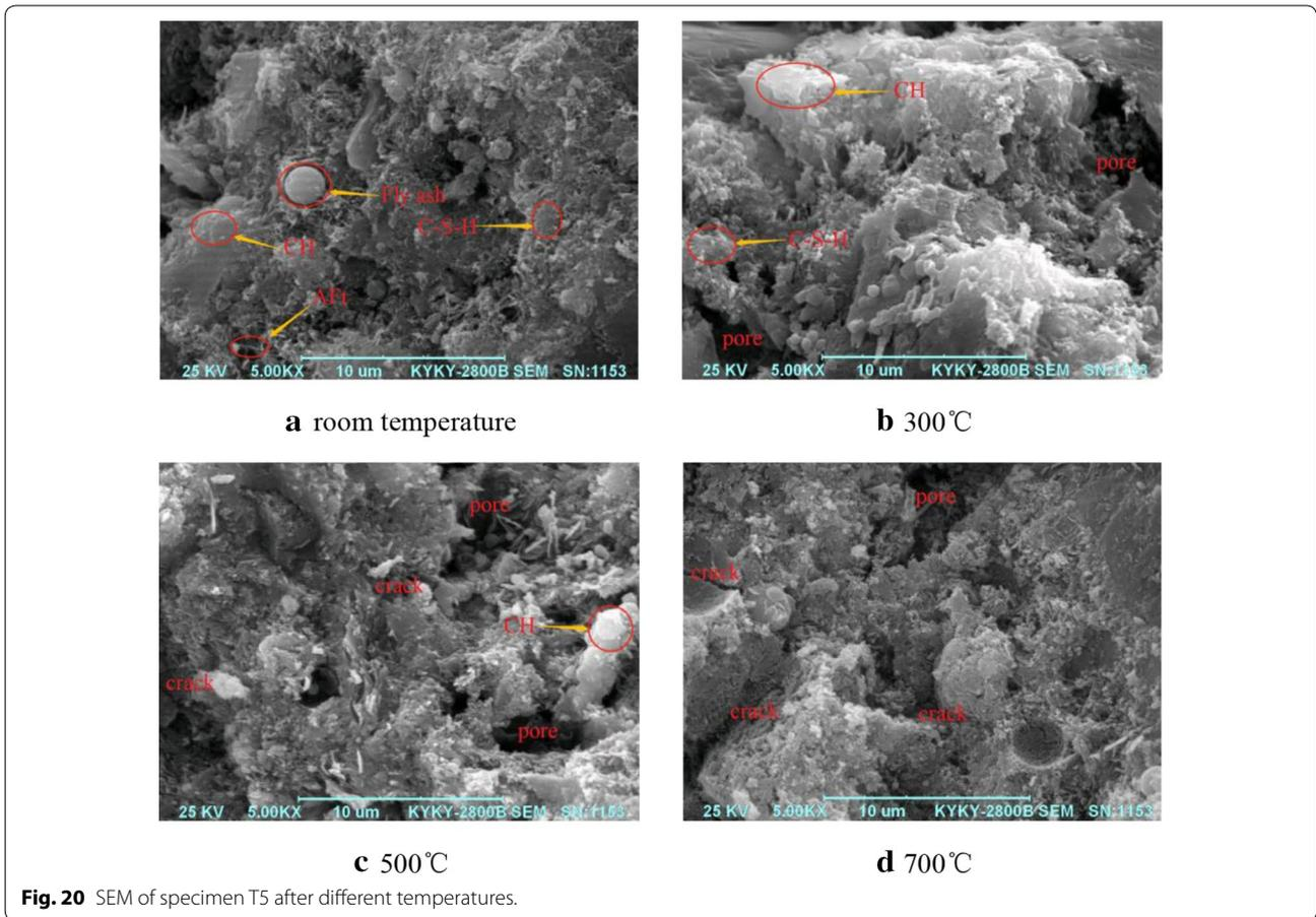
influence of temperature on the microstructure of concrete produced with desert sand, the microscopic experiments (XRD, SEM) were employed. Based on the analysis of experimental results, the major conclusions were summarized in the following.
