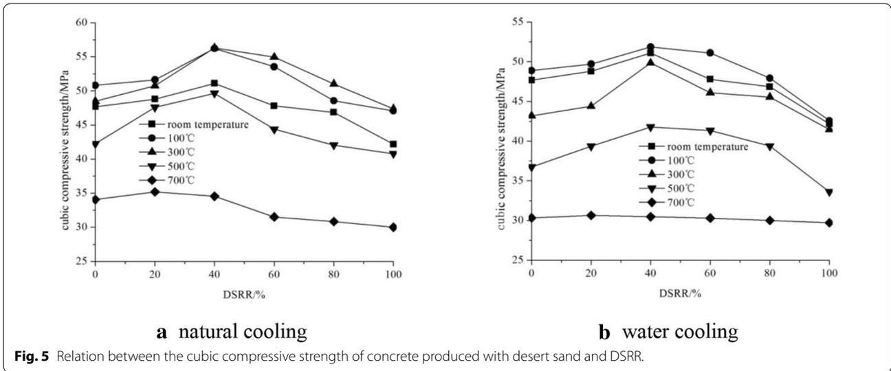
medium sand. So, with the enhancement of DSRR, the cubic compressive strength of concrete produced with desert sand increased firstly, and then declined.
