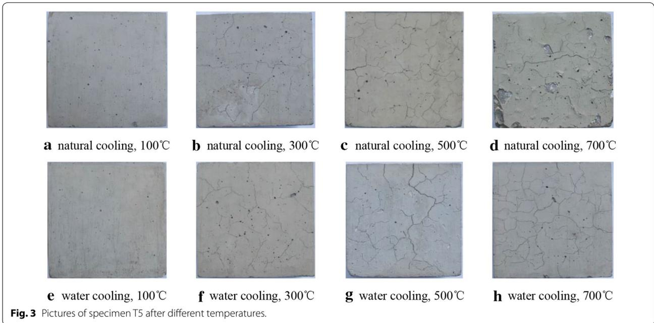
of spalling. Compared with specimen T5 after 500 °C, there were more uniformly distributed micro-cracks on the surface of specimen T5 after 700 °C. Under the condition of water cooling, the appearance of specimens T5 after 100 °C, 300 °C, 500 °C and 700 °C was gray, buff, light yellow and French grey with short capillary crack.
