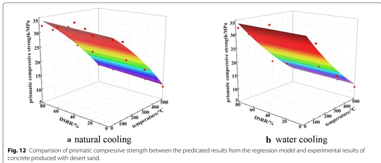
**Fig. 12** Comparison of prismatic compressive strength between the predicated results from the regression model and experimental results of concrete produced with desert sand.
