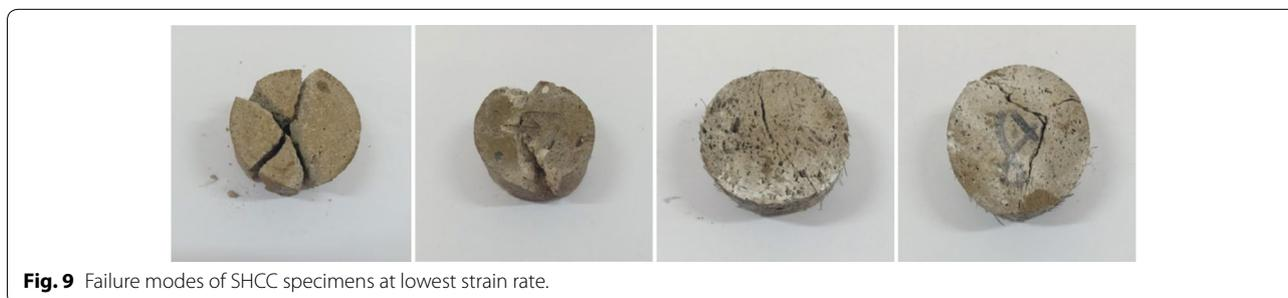
**Fig. 9** Failure modes of SHCC specimens at lowest strain rate.
