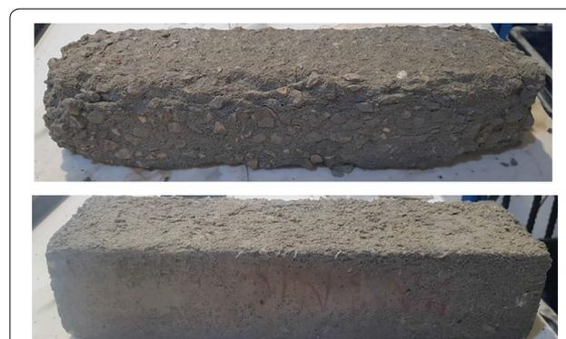
**Fig. 11** View of specimens R20 (top) and R10–H20–T1 (bottom) after 108 cycles.
