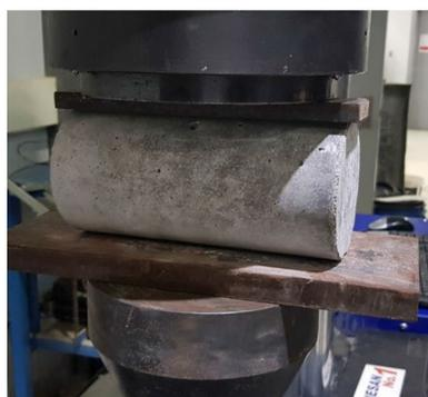
c Splitting tensile strength test.
