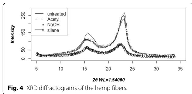
**Fig. 4** XRD diffractograms of the hemp fibers.
