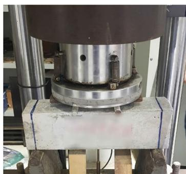
b Flexural strength test.
