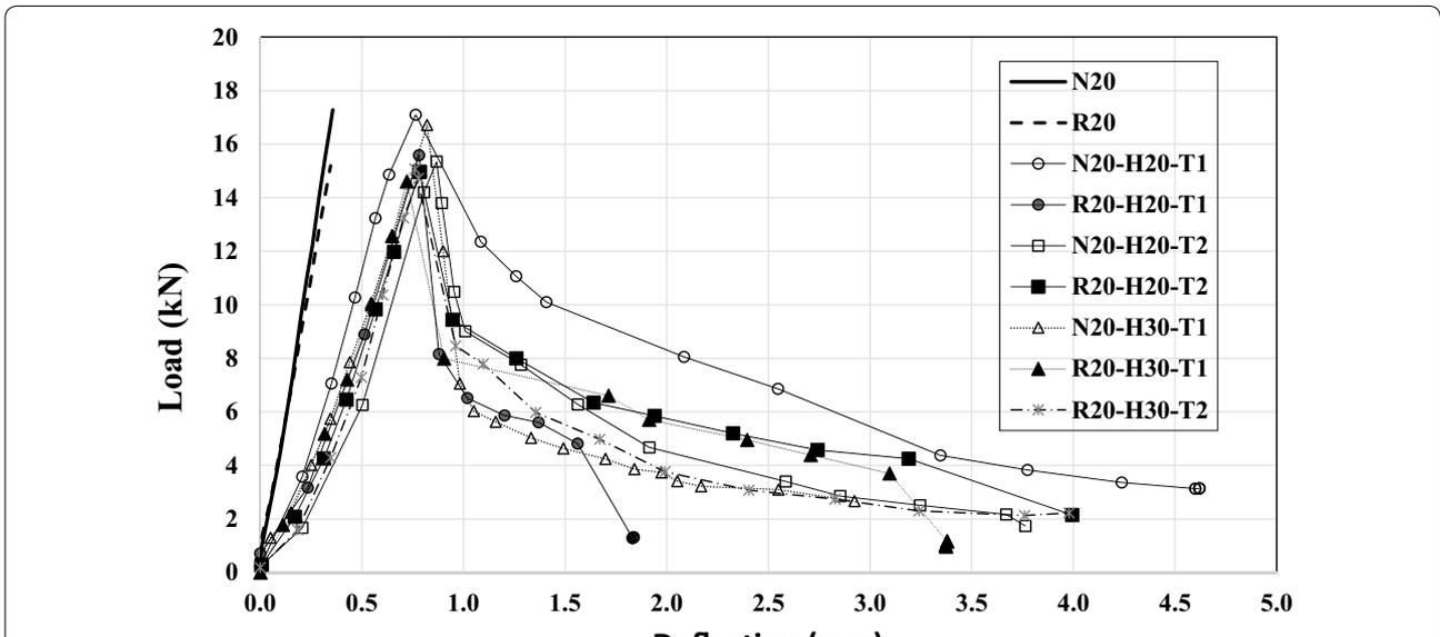
**Fig. 8** Load-deflection curves of the standard beams; Group 2, MSA = 20 mm.
