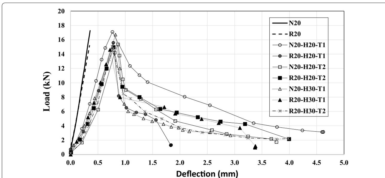
**Fig. 8** Load-deflection curves of the standard beams; Group 2, MSA = 20 mm.
