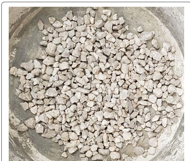
**Fig. 2** Recycled coarse aggregates.
