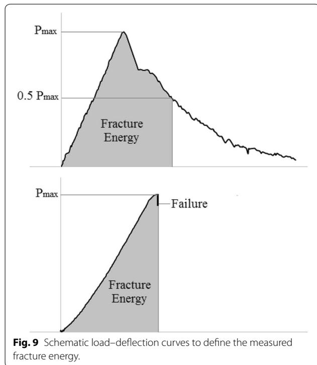
**Fig. 9** Schematic load–deflection curves to define the measured fracture energy.
