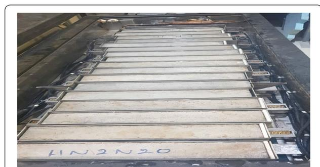
**Fig. 10** View of specimens prepared for freeze thaw cycles.
