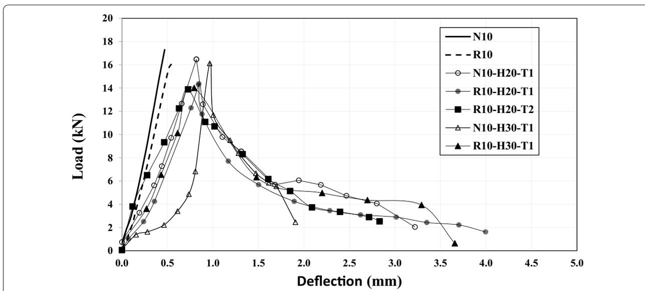
**Fig. 7** Load-deflection curves of the standard beams; Group 1, MSA = 10 mm.
