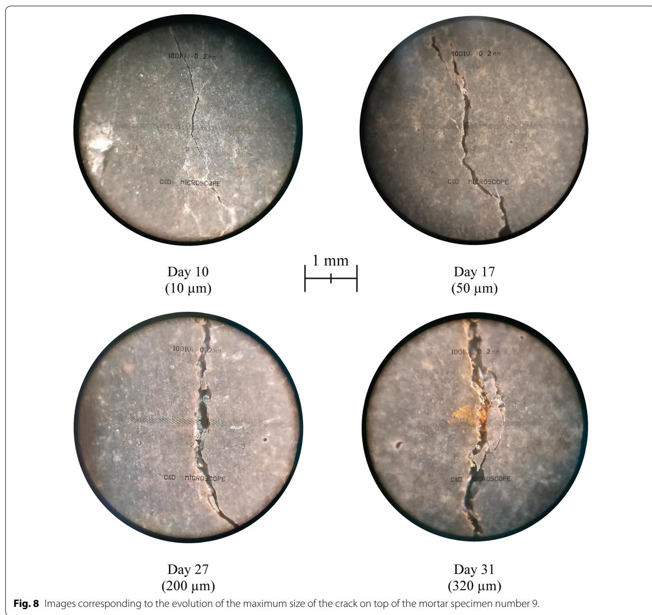
**Fig. 8** Images corresponding to the evolution of the maximum size of the crack on top of the mortar specimen number 9.
