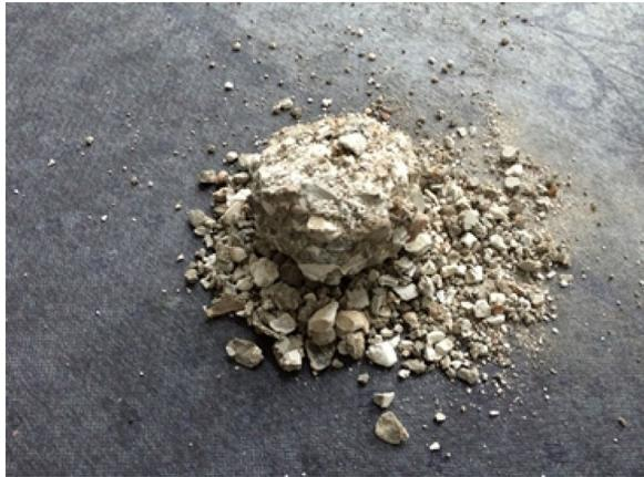
**Fig. 1** The old concrete specimen was damaged when the high temperature was set as 800 °C in the preliminary test.
