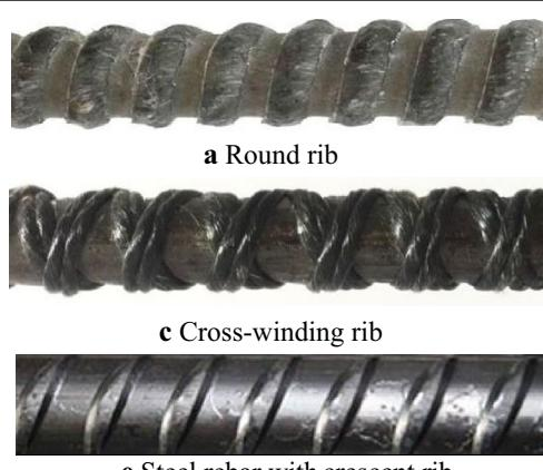
**Fig. 2** Surface shape of rebar.
