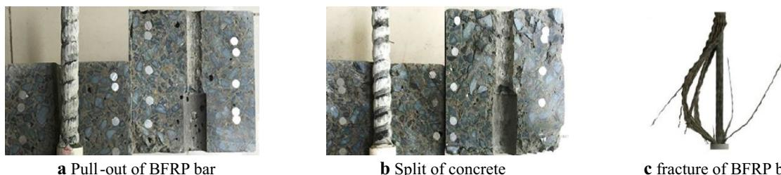
**Fig. 5** Failure modes under cyclic loads.
