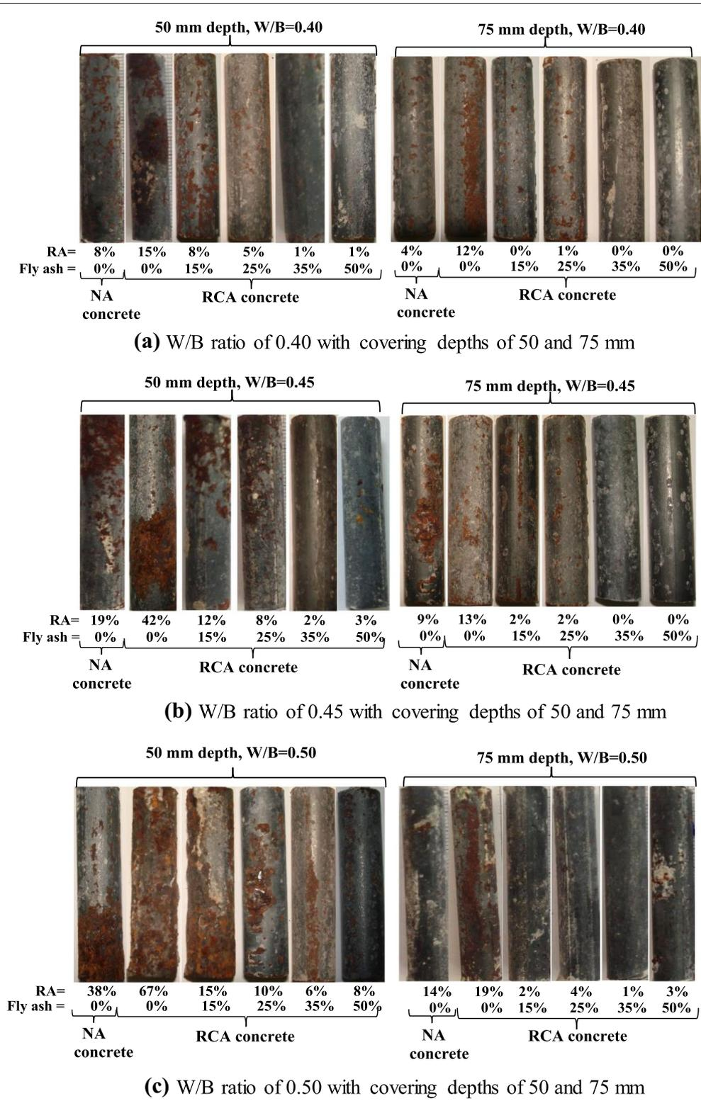
**Fig. 8** Rusted area of embedded steel in NA and RCA concretes with a W/B of **a** 0.40, **b** 0.45 and **c** 0.50 after 7-year exposure in a marine site.
