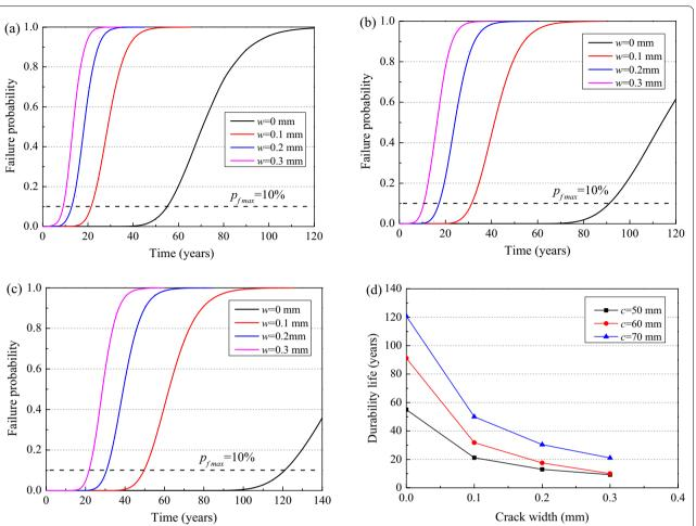
Fig. 9 Effect of cover depth on failure probability: **a** c = 50 mm, **b** c = 60 mm, **c** c = 70 mm and **d** predicted durability life.
