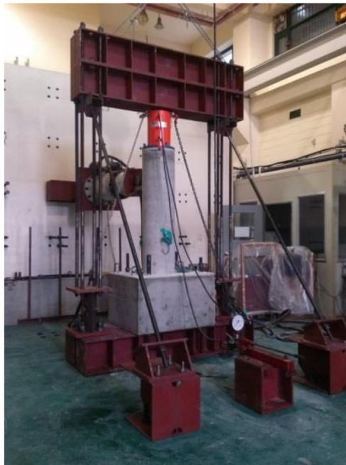
**Fig. 5** Locations of vertical and horizontal loads, strain gauge, and LVDTs and a picture of setup (Note: unit is in mm).
