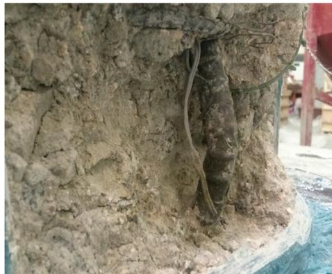
(c) C-1-PET (Bar failed in tension)
