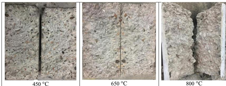
**Fig. 9** Failure modes of fractured surfaces.
