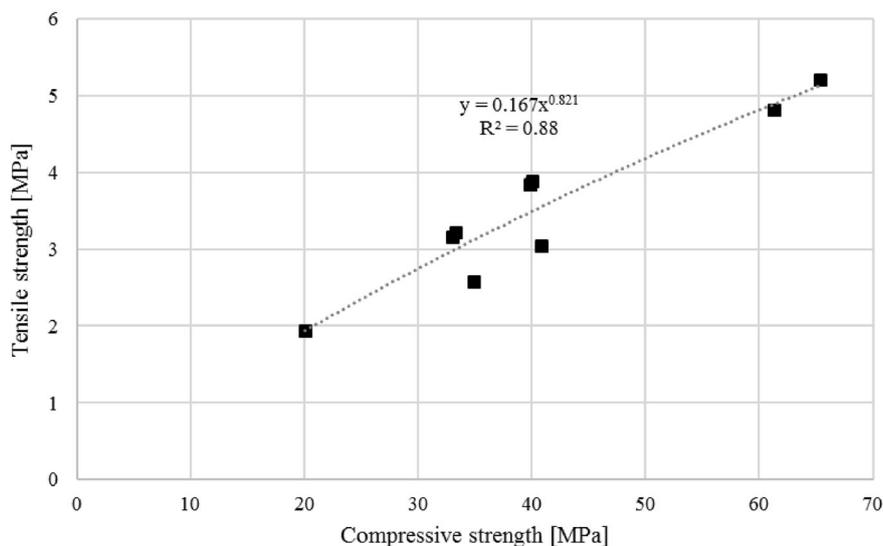
**Fig. 3** Correlation between the tensile strength ( $f_t$ ) and the compressive strength ( $f_c$ ).
