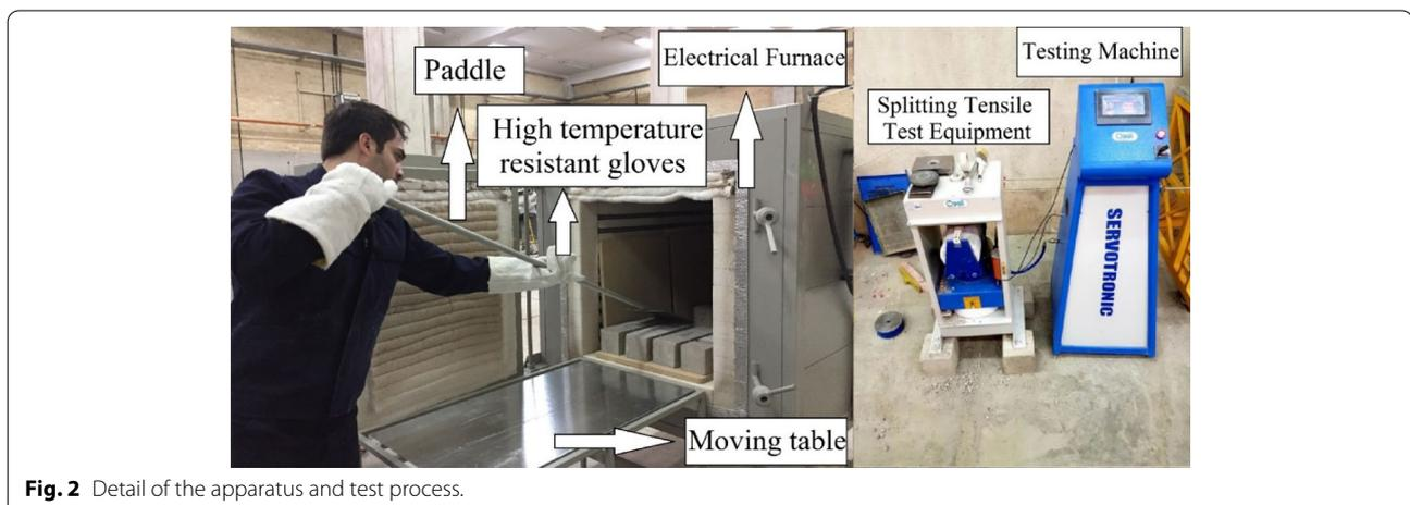
**Fig. 2** Detail of the apparatus and test process.
