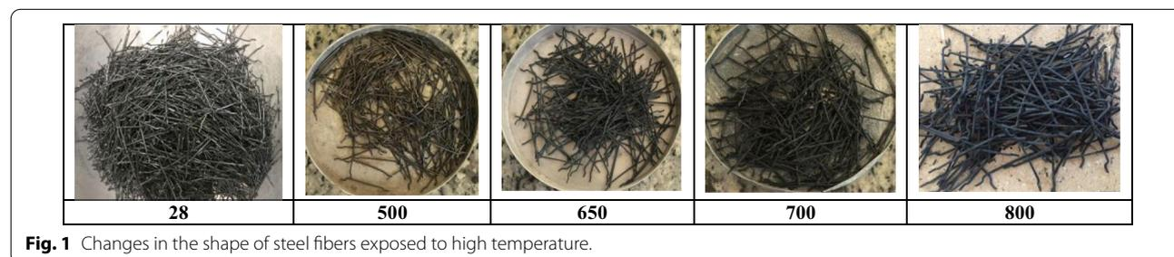
**Fig. 1** Changes in the shape of steel fibers exposed to high temperature.
