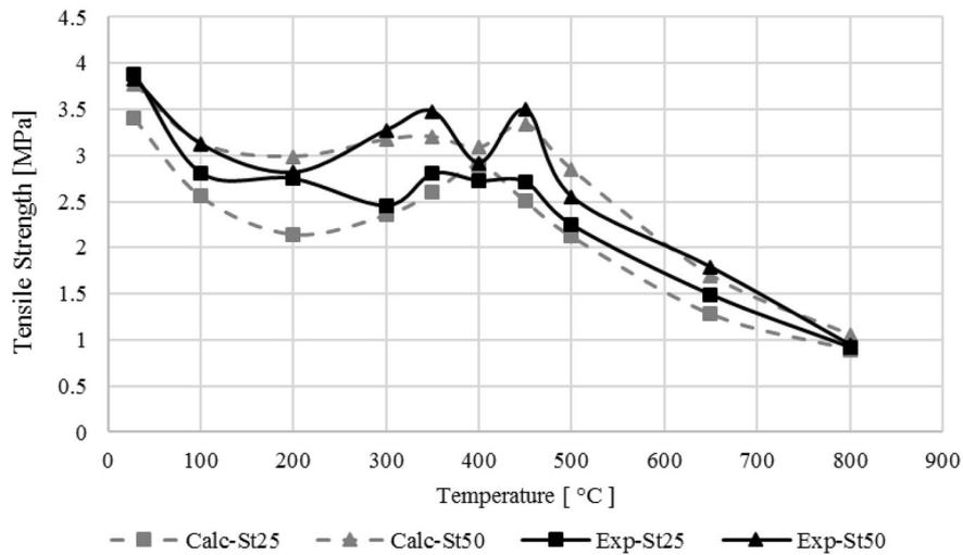
**Fig. 11** Comparison between the predicted tensile strength using Eq. 10 and experimental values.
