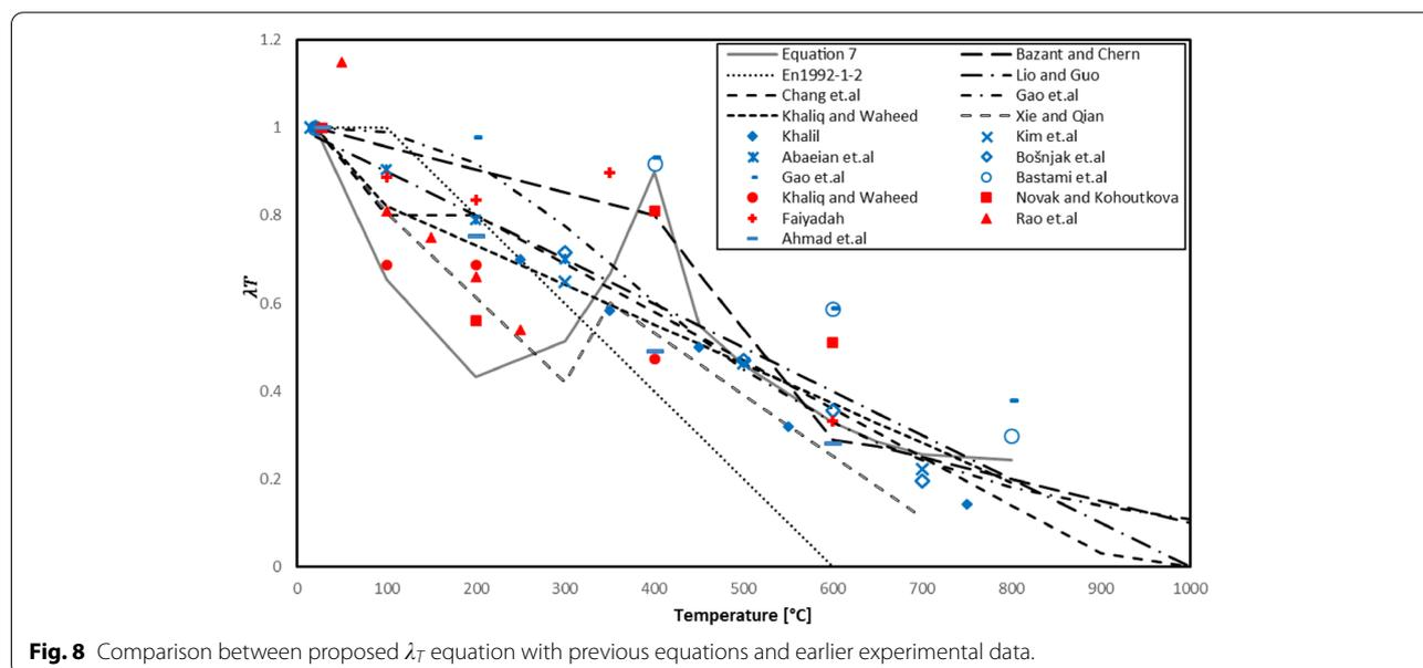
**Fig. 8** Comparison between proposed  $\lambda_T$  equation with previous equations and earlier experimental data.
