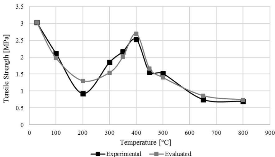
**Fig. 10** Variation of the tensile strength at high temperatures.
