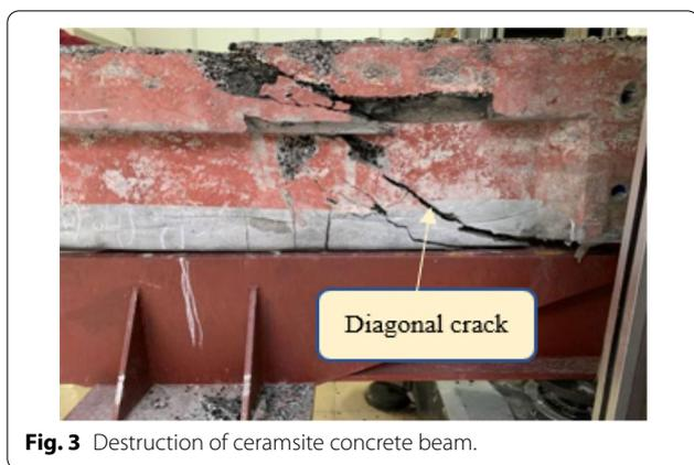
**Fig. 3** Destruction of ceramsite concrete beam.
