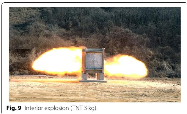
**Fig. 9** Interior explosion (TNT 3 kg).
