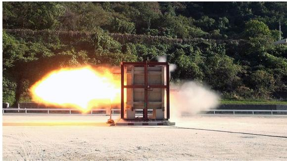
**Fig. 6** Interior explosion (TNT 2 kg).
