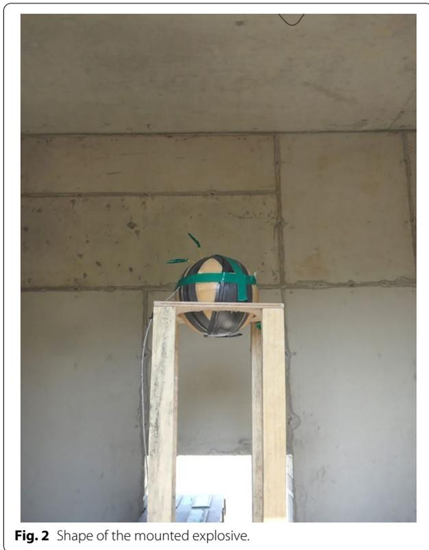
**Fig. 2** Shape of the mounted explosive.
