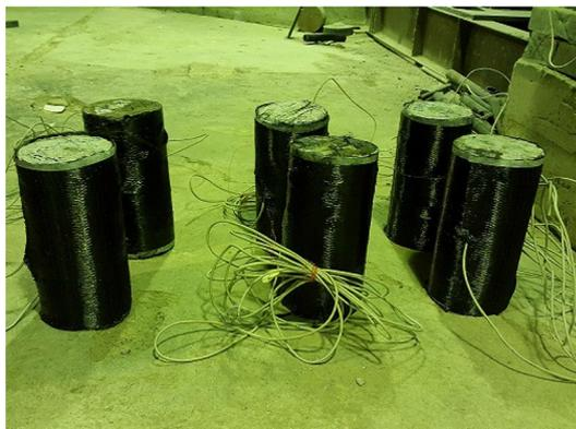
**Fig. 7** CFRP fibers and confined specimens ready for testing compressive strength.
