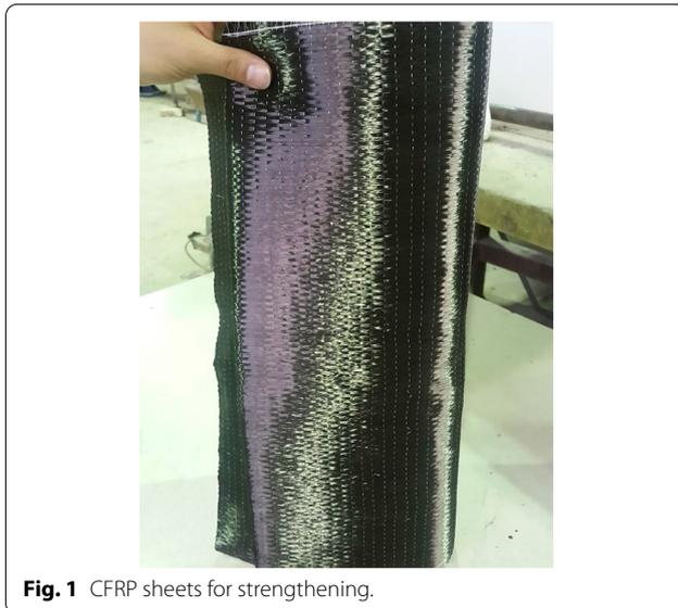
**Fig. 1** CFRP sheets for strengthening.**Table 6** CFRP wraps properties.
