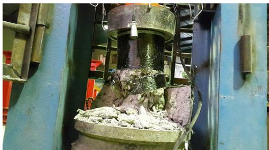
**Fig. 8** Confined specimen with embedded rebar after failure.
