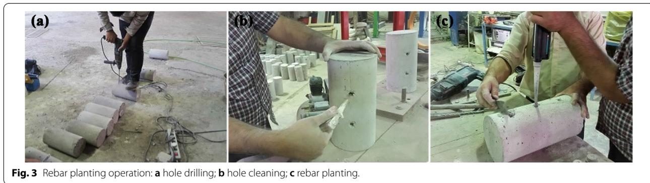
decrease due to the presence of dust and powdered concrete. Special rebar planting adhesive was utilized to plant the rebar specimens in concrete afterward.
