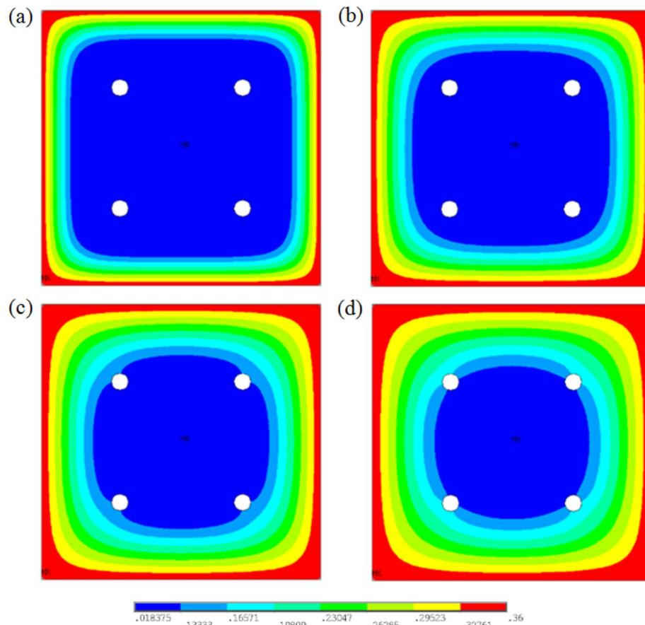
**Fig. 11** Contours of carbon dioxide concentration in the 0.75% PVA fiber concrete component with 6 mm length: **a** for 7 days, **b** for 14 days, **c** for 21 days, and **d** for 28 days.
