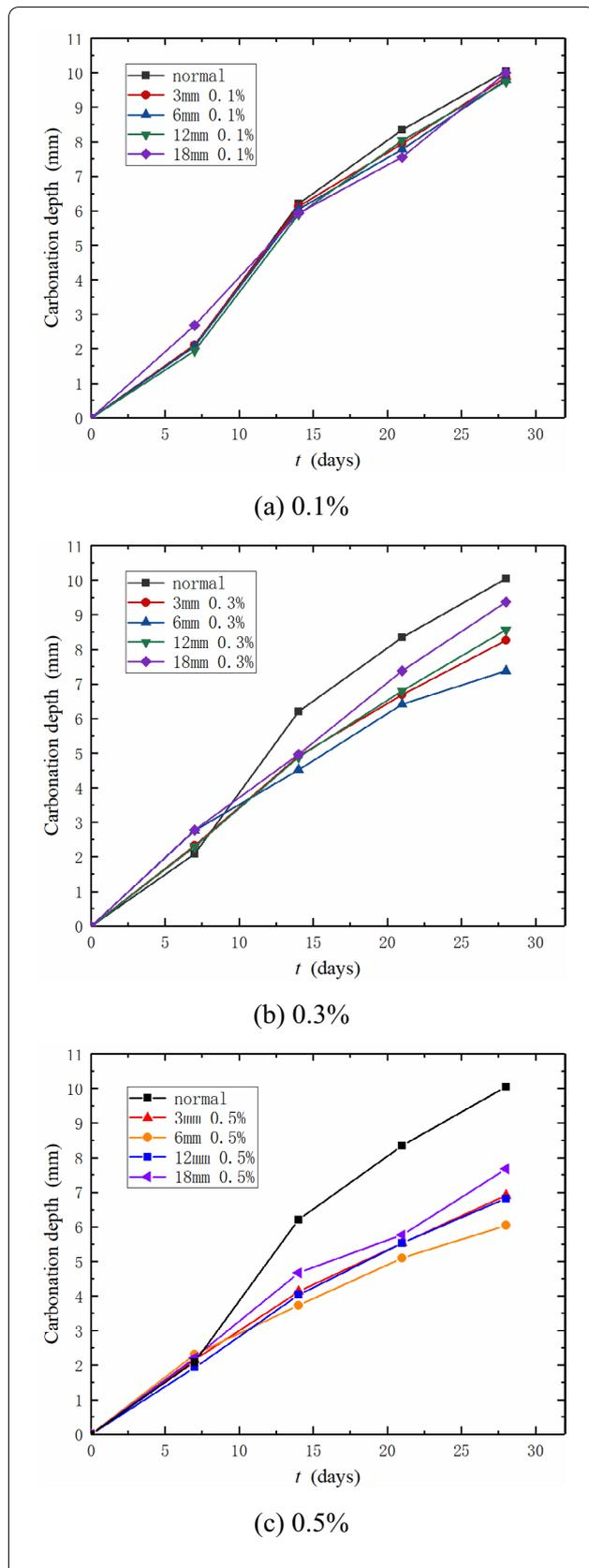
**Fig. 4** Time evolution of carbonation depth in PVA fiber concrete with fiber contents of 0.1%, 0.3% and 0.5%.
