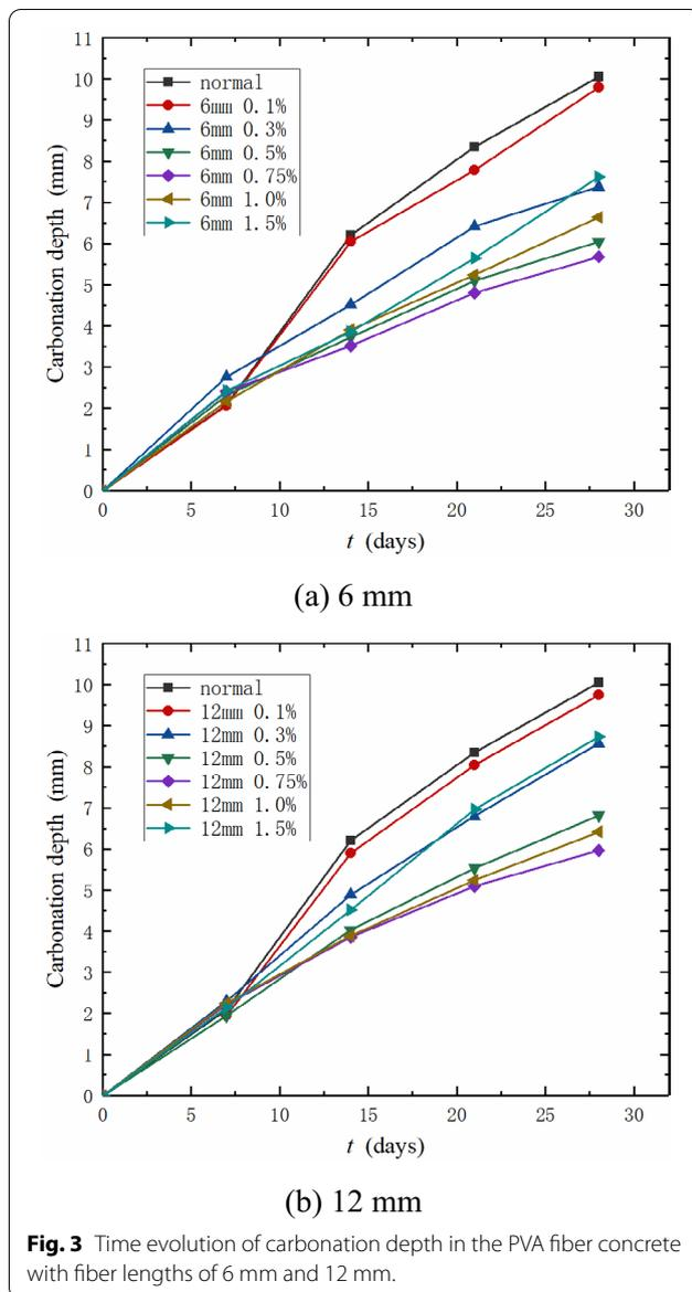
**Fig. 3** Time evolution of carbonation depth in the PVA fiber concrete with fiber lengths of 6 mm and 12 mm.
