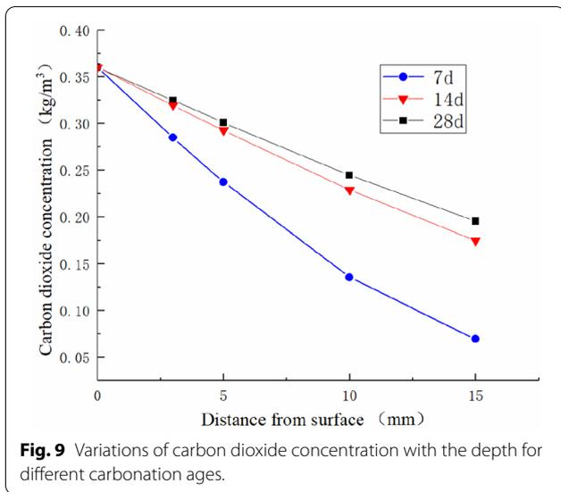
concentration. In addition, the longer the carbonation lasts, the flatter the curve of carbon dioxide concentration is. With the extension of carbonation time, the more fully carbon dioxide diffuses into the component interior, the less the decrease of its concentration with the depth.
