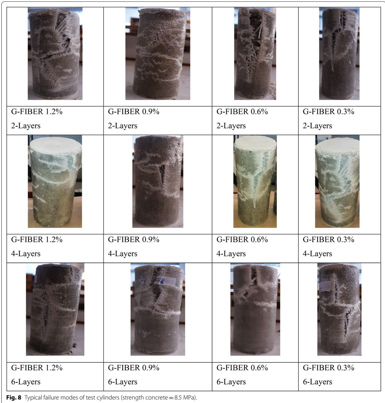
concrete strength equal to 16 MPa, The results indicate an increase in 13% ,18%,20% and 20% for models Gher-nouti et al. (2011), Bensaid et al. (2010), AL-Salloum et al. (2007) and Teng et al. (2007) respectively. For concrete strength equal to 8.5 MPa, The results indicate an increase in 54% ,60%,65% and 70% for models Gher-nouti et al. (2011), Bensaid et al. (2010), AL-Salloum et al. (2007) and Teng et al. (2007) respectively. Although the
