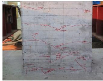
(a) Cracks on the back side
