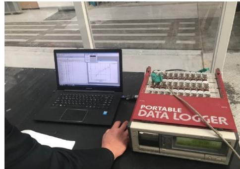
(a) Concrete static strain measuring equipment (TDS-303)
