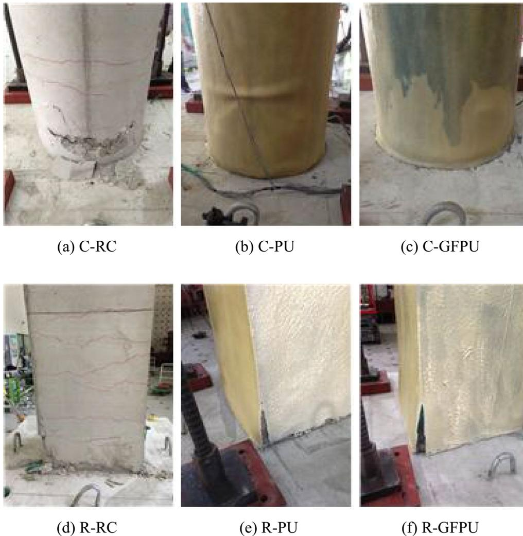
**Fig. 22** Failure behavior of specimens of pseudo-dynamic test.
