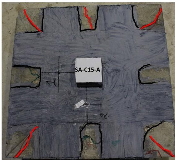
(a) Failure of specimen SA-C15-A
