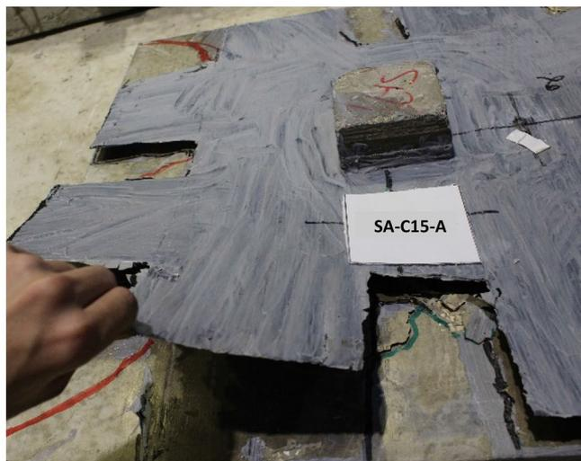
(b) Debonding of CFRP sheets in SA-C15-A
