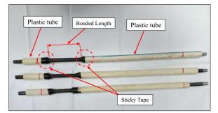
Fig. 3 Shape of tested rebars before placing in the mold
