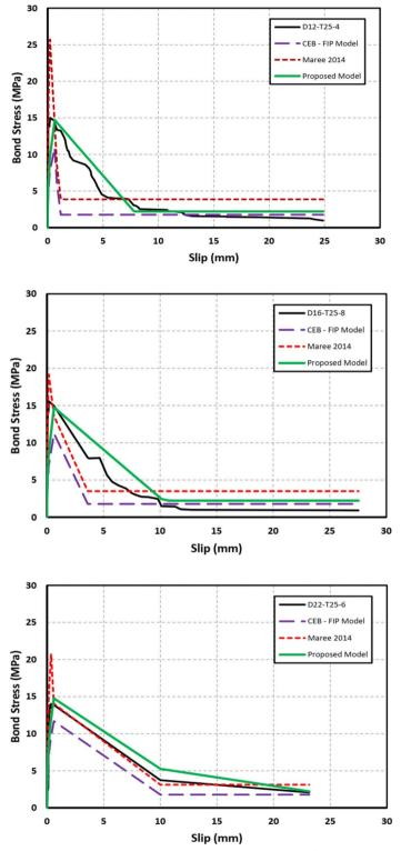
Fig. 23 Proposed analytical versus experimental bond-slip relationships (ambient temperature of 25 °C)
