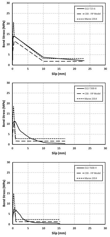
Fig. 22 Analytical versus experimental bond-slip curves (specimens of 22-mm-diameter rebars)
