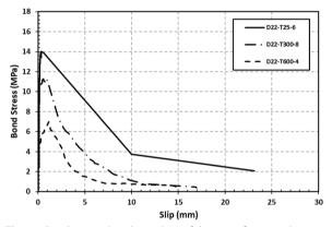
Fig. 16 Bond stress–slip relationships of the case of 22-mm-diameter rebars
