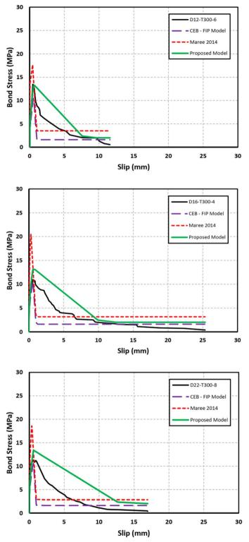
Fig. 24 Proposed analytical versus experimental bond-slip relationships (elevated temperature of 300 °C)
