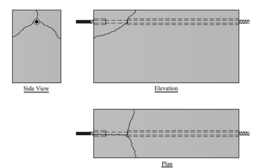
Fig. 12 Typical cracking pattern of the tested beam-end specimens
