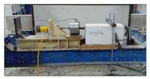
Fig. 6 Setup of beam-end specimen test
