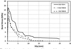
Fig. 14 Bond stress–slip relationships of the case of 12-mm-diameter rebars
