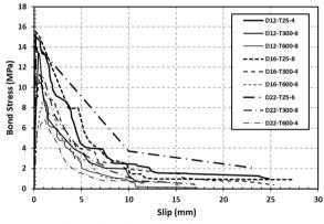
Fig. 13 Bond stress-slip relationships of all test specimens
