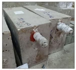
(b) Beam-end specimens after covering the rebars with the heat-insulation material.
