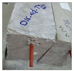
(a) Beam-end specimens after painting the rebars with the anti-rust material.
