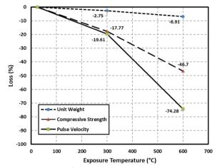
Fig. 10 Percentage of unit weight loss, compressive strength loss and ultrasonic-pulse velocity loss for all extracted specimens
