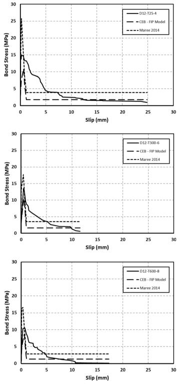
Fig. 20 Analytical versus experimental bond-slip curves (specimens of 12-mm-diameter rebars)
