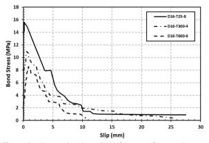
Fig. 15 Bond stress–slip relationships of the case of 16-mm-diameter rebars
