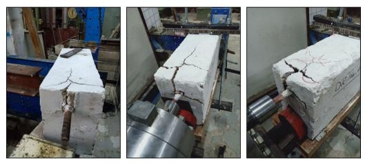
D22-T25-6 D22-T300-8 Fig. 11 Modes of failure and cracking patterns for all tested beam-end specimens
