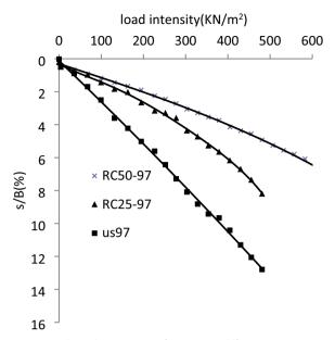
Fig. 10 Load settelment curves of mixtures at differnet RC (Dr = 97%)
