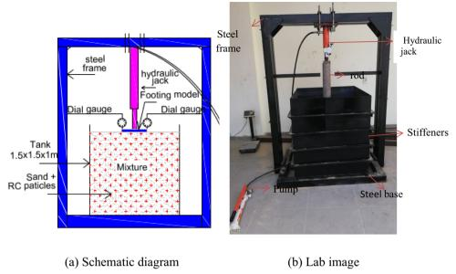
Fig. 3 Testing setup
