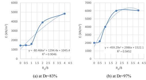
**Fig. 24** Effect of  $R_d/B$  on E & RC = 25%
