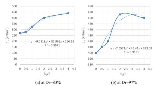
**Fig. 23** Effect of  $R_d$  on the  $q_u \& RC = 25\%$
