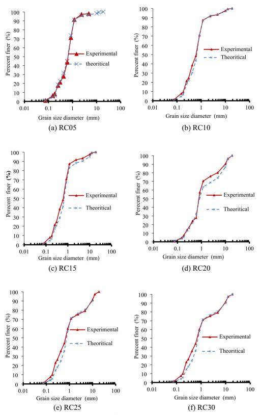
Fig. 4 Experimental and theoritical grain size distribution curves of tested samples
