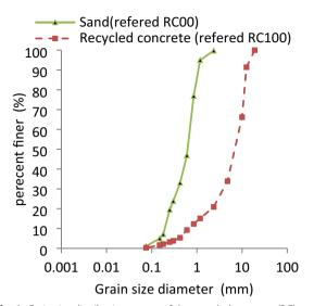
**Fig. 1** Grain size distribution curves of the recycled concrete (RC) and unreinforced (pure) sand (US), RC is labeled RC100 and US is denoted by RC00
