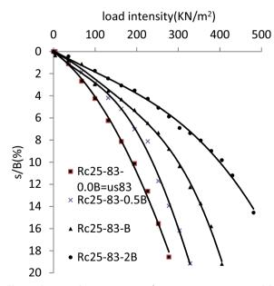
Fig. 12 Stress-settlement response of mixture incorporating 25% RC at different  $R_d$  (0B, 0.5B, B and 2B), Dr = 83%
