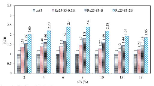
Fig. 14 BCR change with s/B at different  $R_d$  for Dr = 83%
