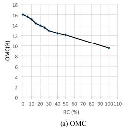
Fig. 7 RC content vs OMC and MDD for all tested samples
