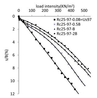
**Fig. 13** Stress-settlement response of mixture incorporating 25% RC at different  $R_d$  (0B, 0.5B, B and 2B), Dr = 97%
