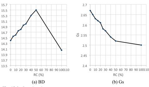
Fig. 5 RC content vs BD and Gs for all tested samples
