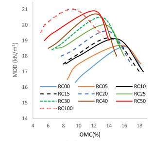
Fig. 6 Compaction curves for all presented mixes incorporating different levels of RC
