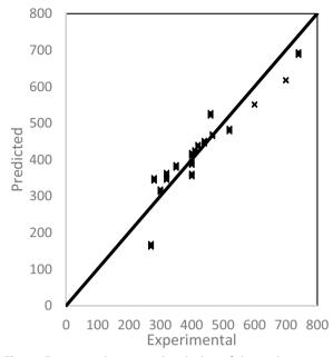
Fig. 25 Experimental versus predicted values of ultimate bearing capacity  $\left( q_{u}\right)$
