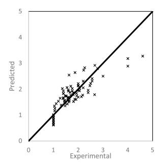
Fig. 27 Experimental versus predicted values of bearing capacity ratio (BCR)
