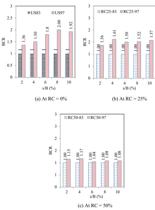
Fig. 18 Effect of Dr on BCR at different RC content (0, 25 and 50%)
