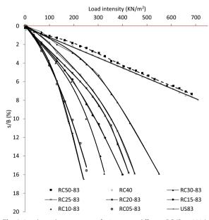
Fig. 8 Load settelment curves of mixtures at differnet RC (Dr = 83%)
