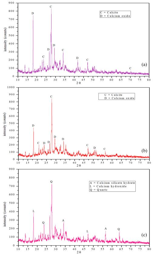
Fig. 14 XRD analysis of concrete made with a B. flexus, b S. koreensis, c no bacteria
