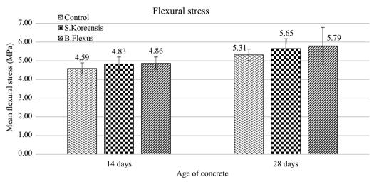
Fig. 4 Flexural strength test result
