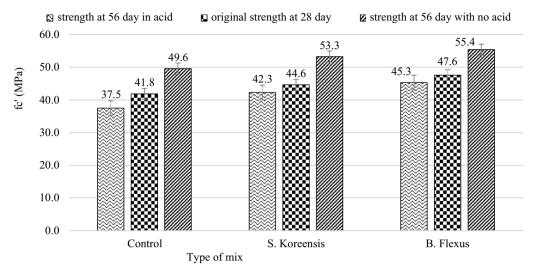
(a) Comparison for compressive strength of concrete exposed to acid
