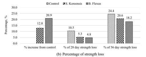
Fig. 8 Comparison of compressive strength of concrete exposed to acid
