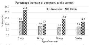
Fig. 3 Percentage increase in compressive strength as compared to the control
