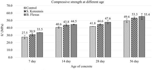
Fig. 2 Compressive strength of concrete at different age
