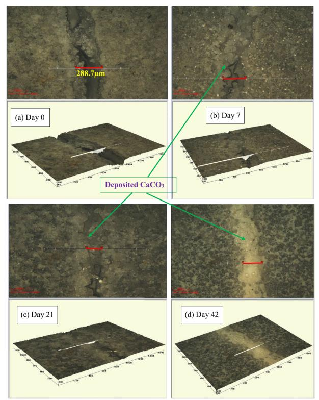
Fig. 12 Self-healing progress of concrete specimen S. koreensis 2 at the age of a 0 day, b 7 days, c 21 days d 42 days
