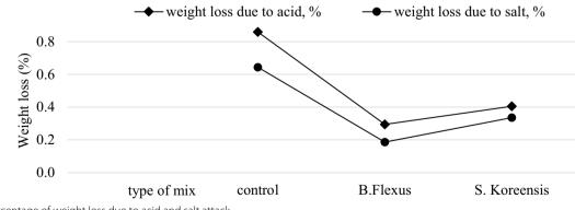
Fig. 9 Percentage of weight loss due to acid and salt attack
