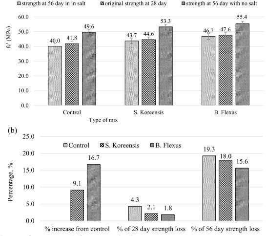
(a) Comparison for compressive strength of concrete exposed to Salt
