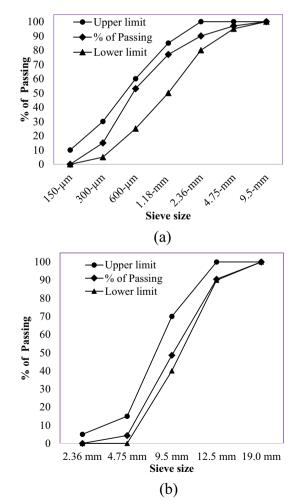
Fig. 1 Gradation of a fine aggregate b coarse aggregate
