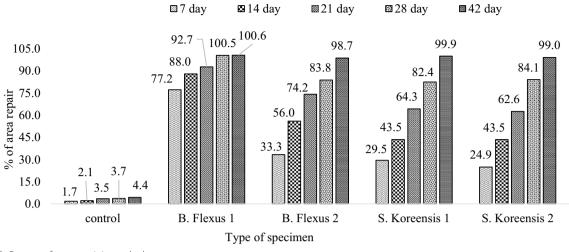
Fig. 13 Percent of area repair in cracked concrete
