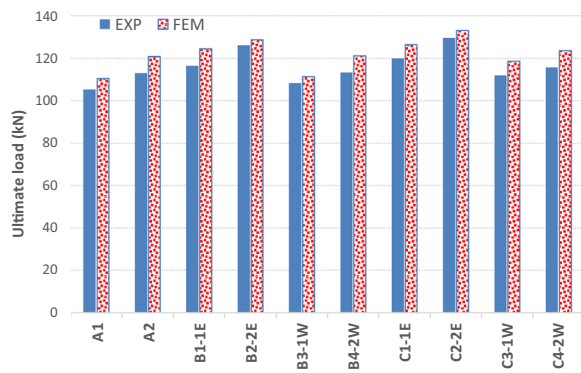
Fig. 18 Comparison between Exp. ultimate load and NLFE ultimate load
