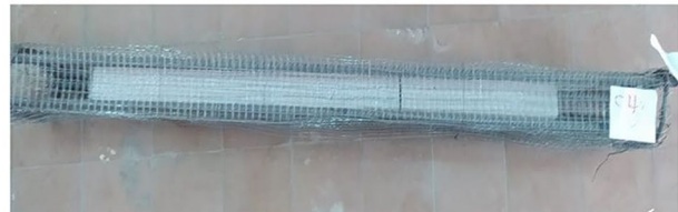
m) Two Layers of Welded Wire Mesh (C4).
