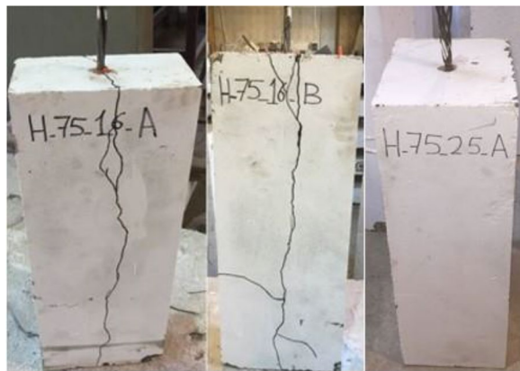
Fig. 6 Effect of increasing slab thickness on improving crack propagation in "H" specimens
