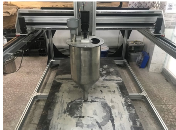
Fig. 5 The gantry concrete printer used in the actual printing test
