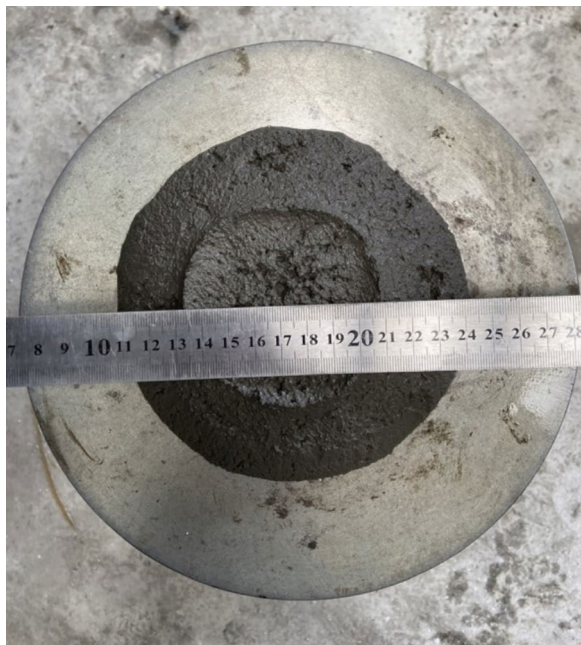
Fig. 3 Measurement of slump flow value of 3D-printed concrete using SA
