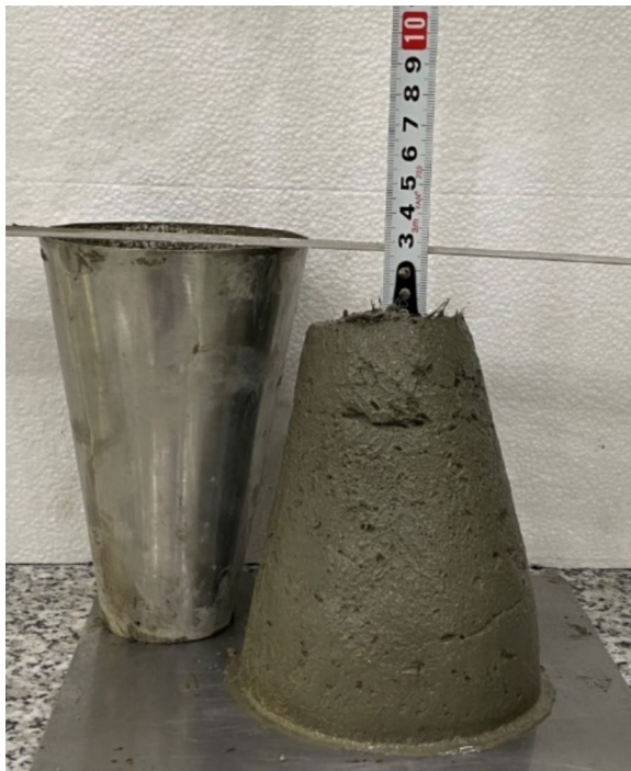
Fig. 2 Measurement of slump value of 3D-printed concrete using SA
