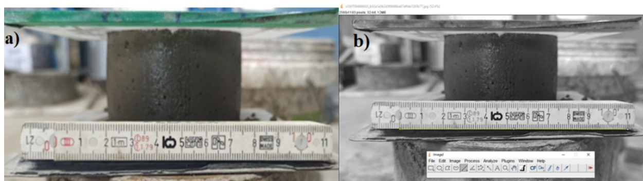
Fig. 6 a Cylinder stability test setup, b analyzing images utilizing ImageJ software
