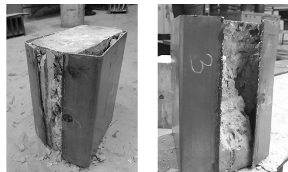
Fig. 9 Example of cold-formed steel splitting accompanied with crushing failure of the confined concrete specimens
