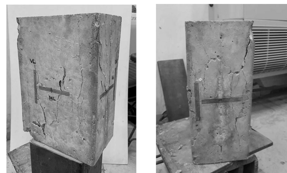
Fig. 8 Example of crushing failure of the unconfined concrete specimens
