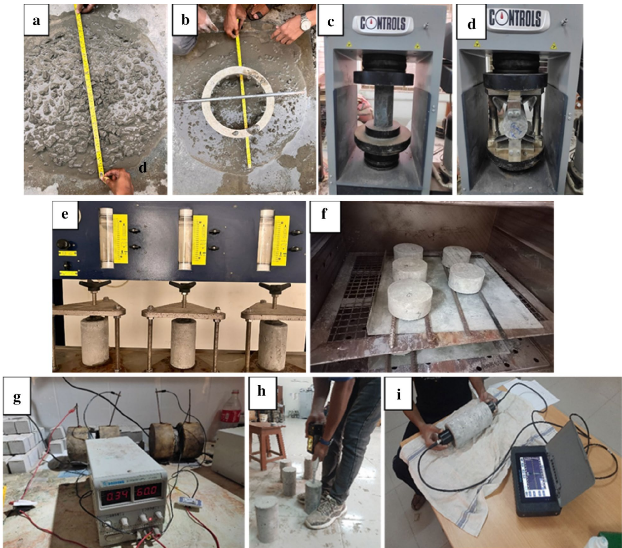
Fig. 2 Test setup on HSSCC of (a) slump flow (b) J-ring flow (c) compressive strength (d) splitting tensile strength (e) water permeability (f) sorptivity (g) RCPT (h) rebound hammer and (i) UPV assessment
