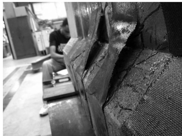
Fig. 12 Debonding at angle of IB-05.
