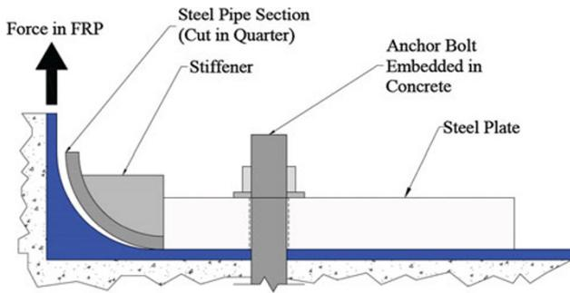
Fig. 13 Anchorage system studied in Grelle (2011).
