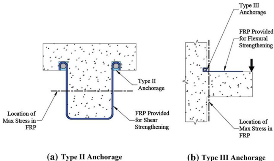
Fig. 3 Comparison of Type II and Type III anchorage (U-Anchor example).
