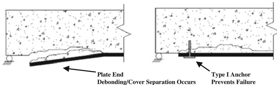
Fig. 2 Example of Type I anchorage device.
