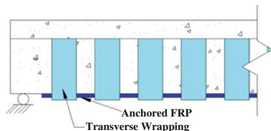
Fig. 5 Example of transverse wrapping anchorage on T-beam.
