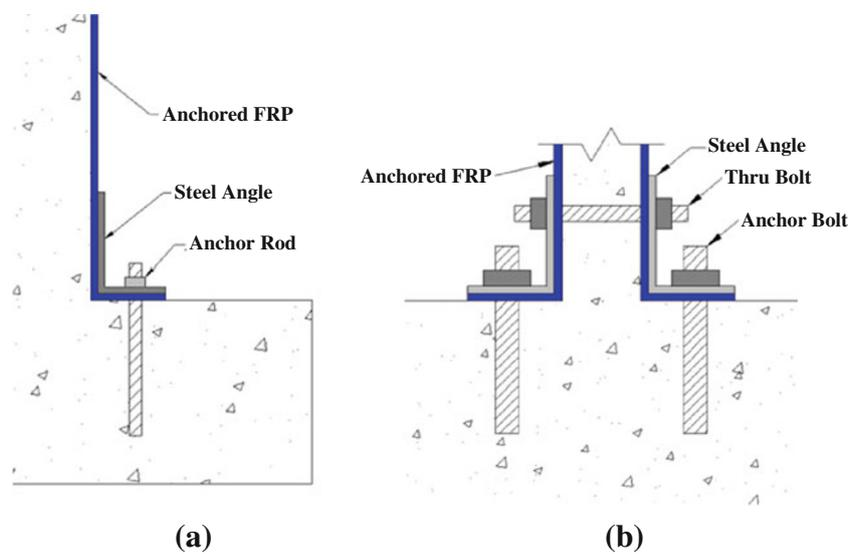
Fig. 10 Bolted angle systems.
