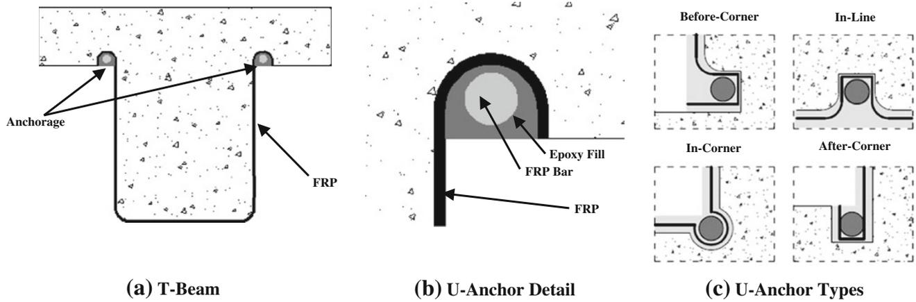
Fig. 6 Schematic of typical U-Anchor (Grelle and Sneed 2011).
