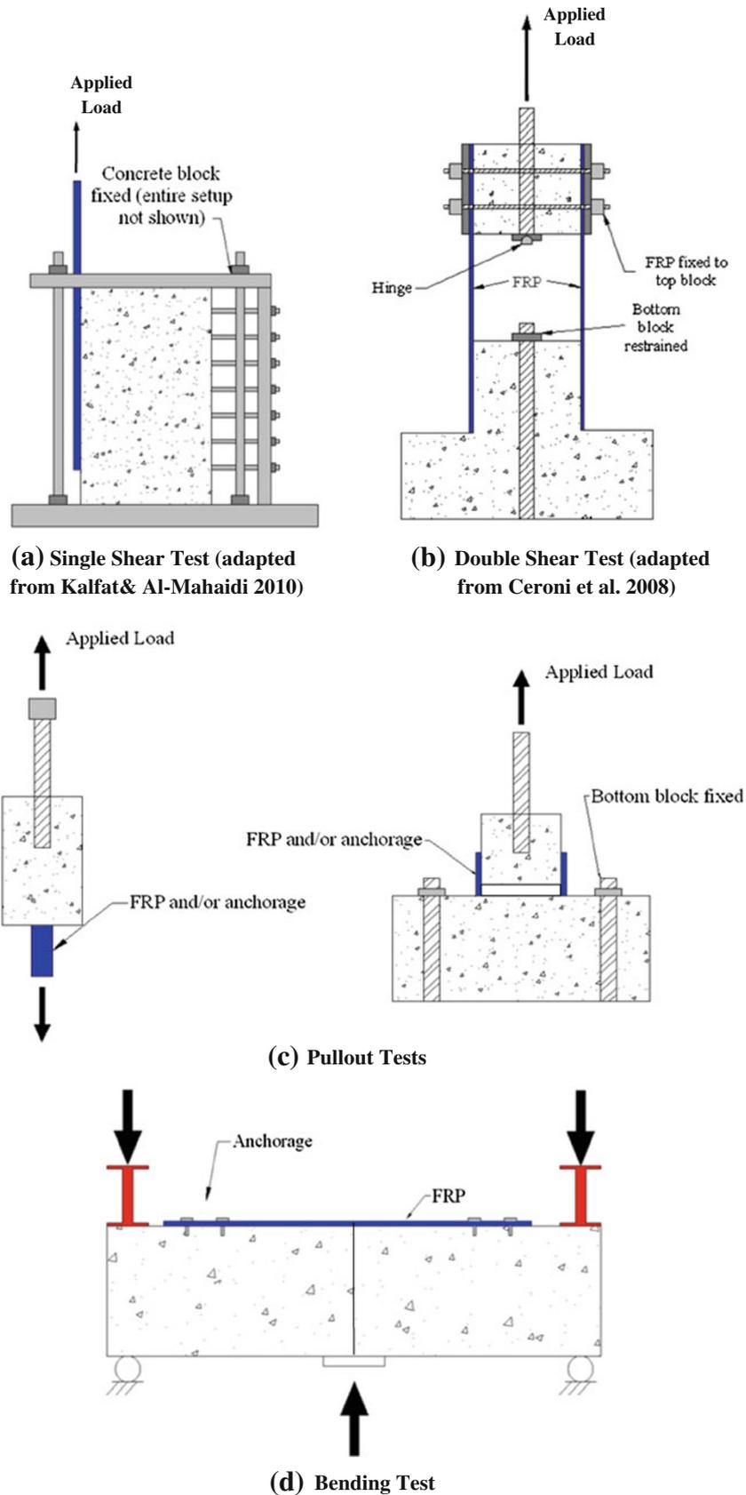
Fig. 15 FRP anchorage testing types.
