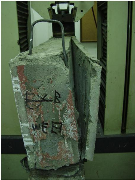
Fig. 11 Separation of the side of the ferrocement form from the brick core for beams of group 4.
