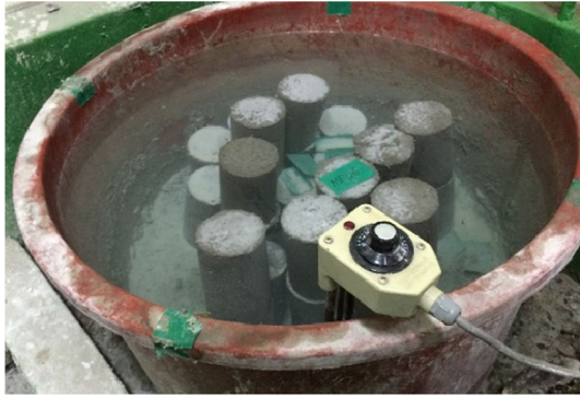
Fig. 3 Curing specimens following ASTM C31.
