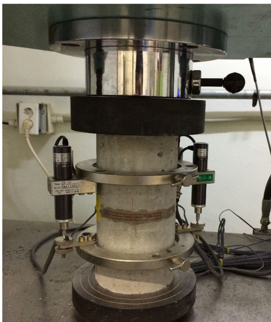
Fig. 4 Test setup for cylindrical specimens.
