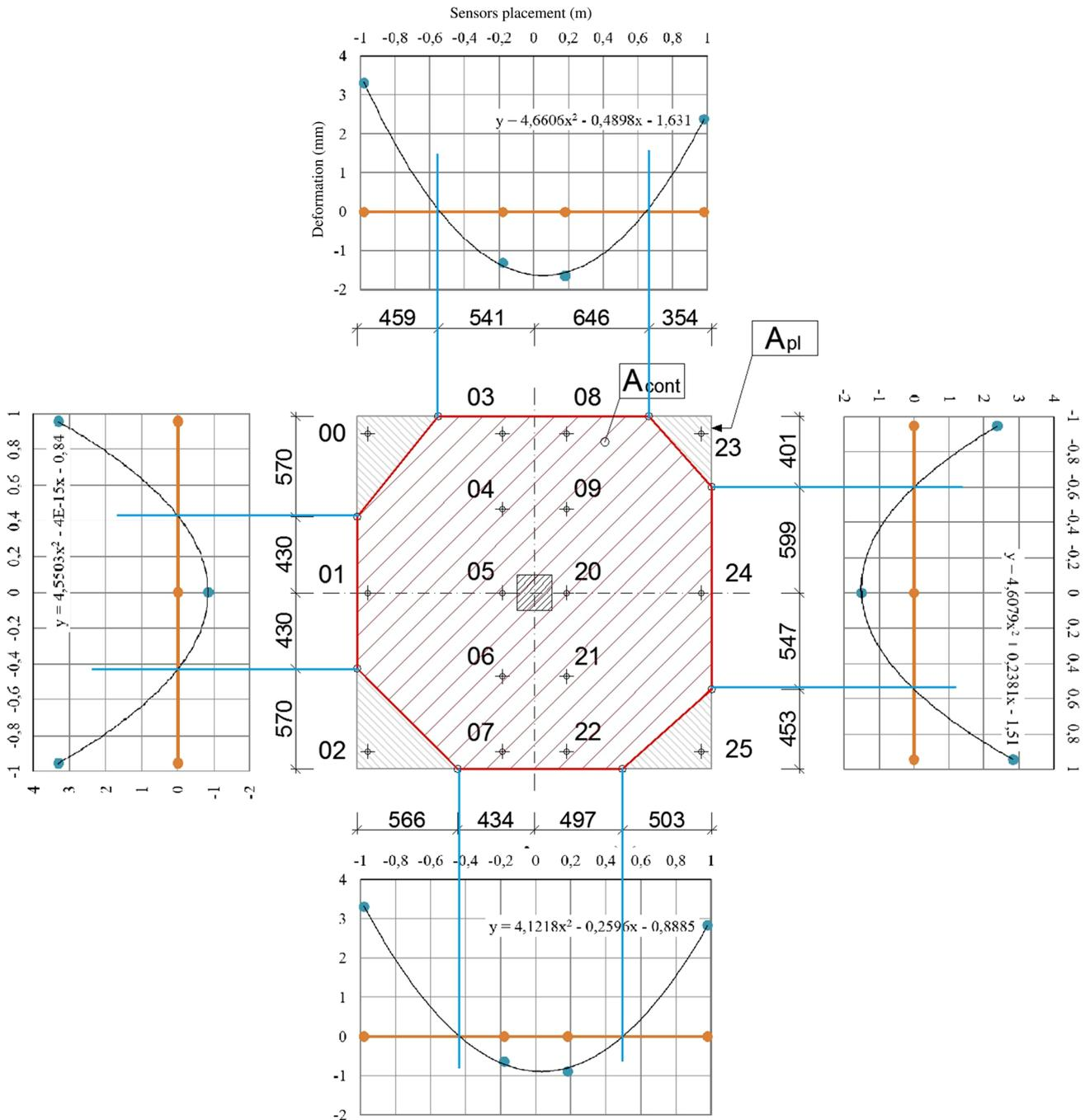
Fig. 11 Analysis of contact surface after step 5.
