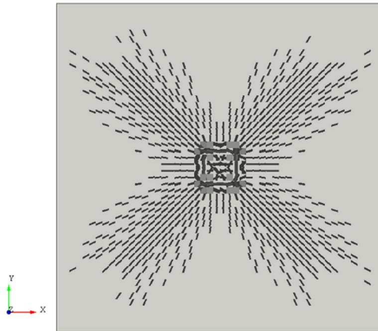
Fig. 13 Cracked slab: standard values for concrete and  $E_{def}$  33.86 MPa.
