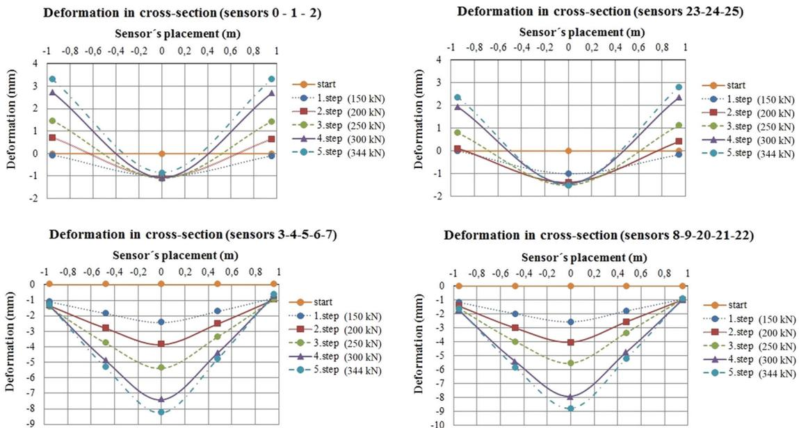
Fig. 5 Vertical deformation of the slab—in cross-sections (mm).
