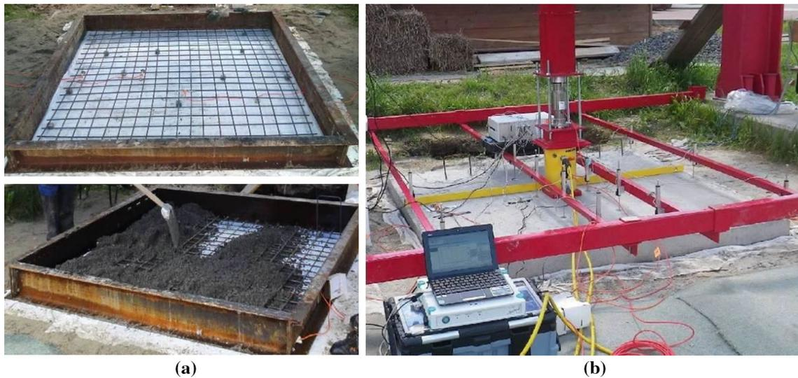
**Fig. 3** Concreting of the slab model and loading test. **a** Concreting of the slab and **b** Loading test
