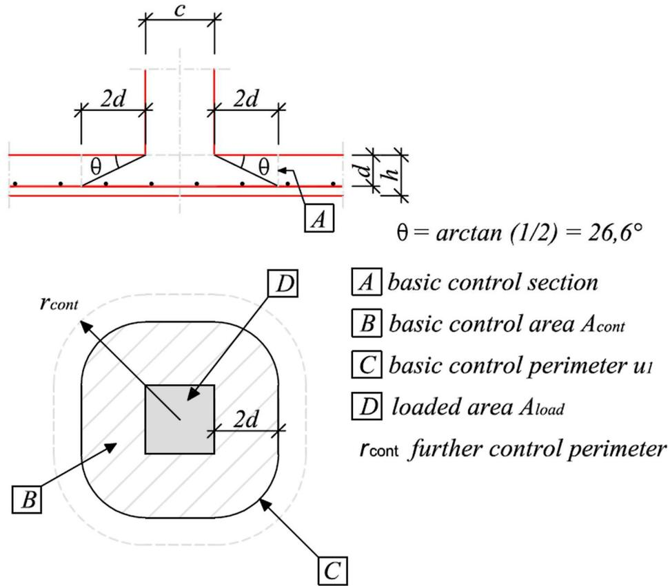
Fig. 1 Verification model for punching shear at the ultimate limit state.
