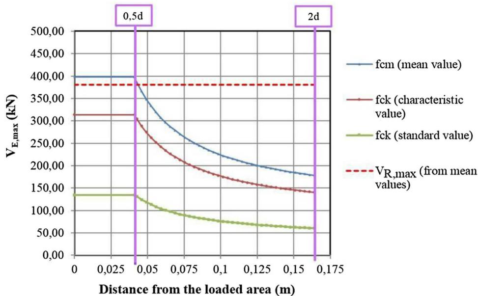
**Fig. 10** Maximum punching shear force according to EC2.
