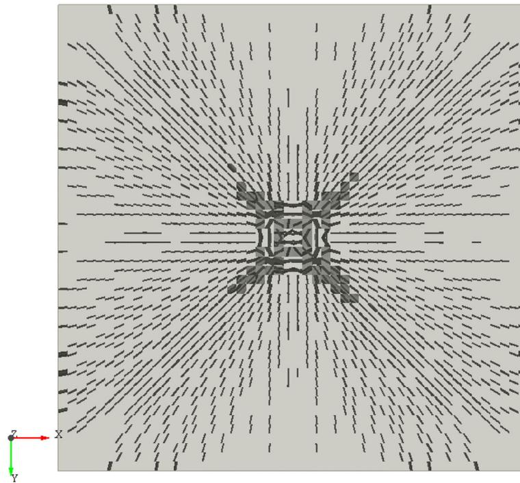
**Fig. 14** 3D cracked slab: standard values for concrete and  $E_{def}$  33.86 MPa.
