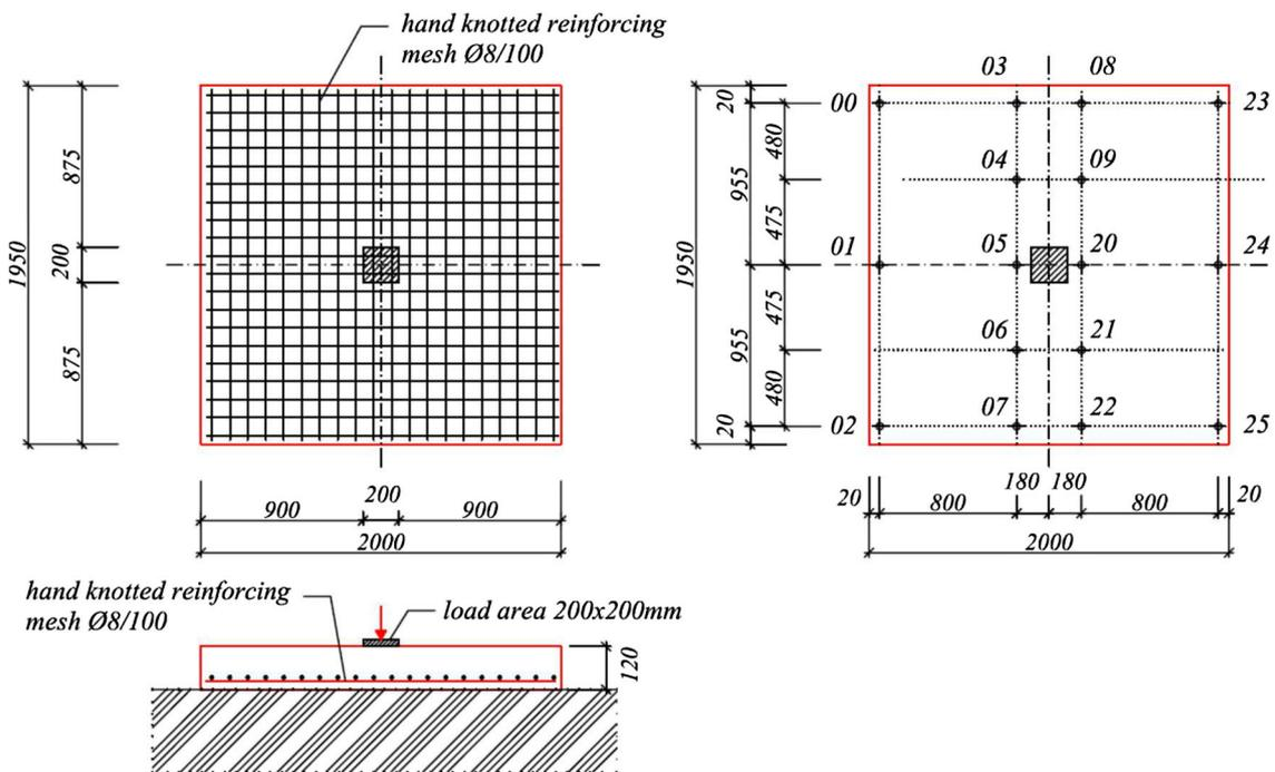
Fig. 2 The test sample and placement of deformation sensors (mm).
