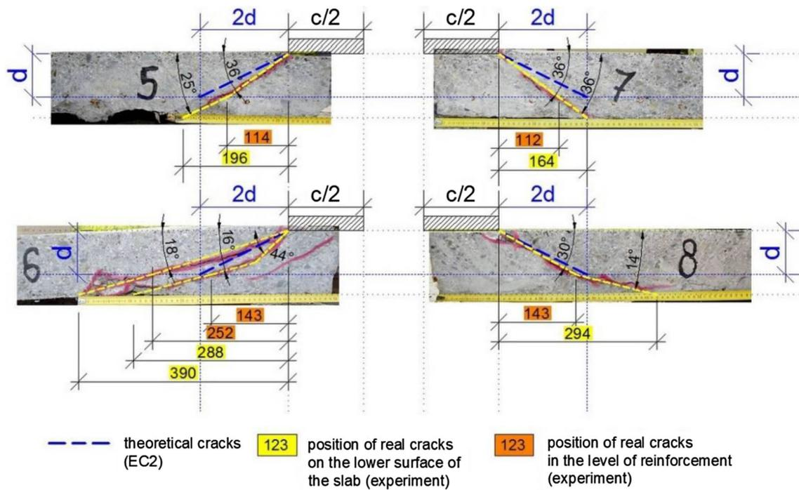
**Fig. 9** Comparison of the measured values and the results of the design methods used in EC2 in diagonal cuts of the slab (mm).
