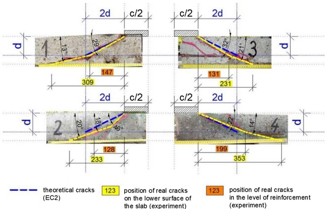
Fig. 8 Comparison of the measured values and the results of the design methods used in EC2 in lateral cuts of the slab (mm).
