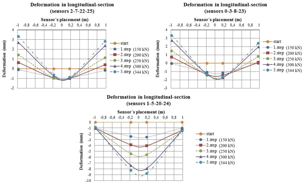
Fig. 6 Vertical deformation of the slab—in longitudinal-sections (mm).
