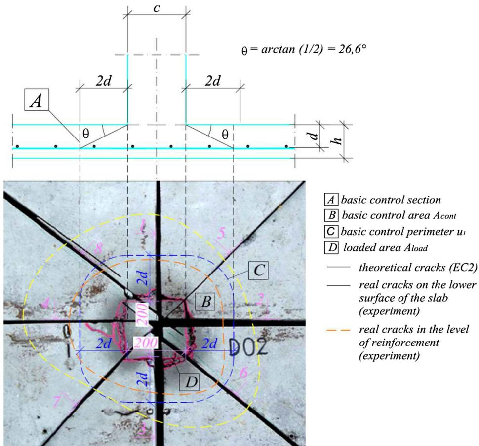
Fig. 7 Verification model for punching shear at the ultimate limit state (mm).
