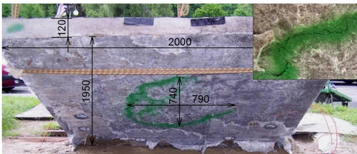
**Fig. 4** Cracks on the bottom surface of the slab (mm).
